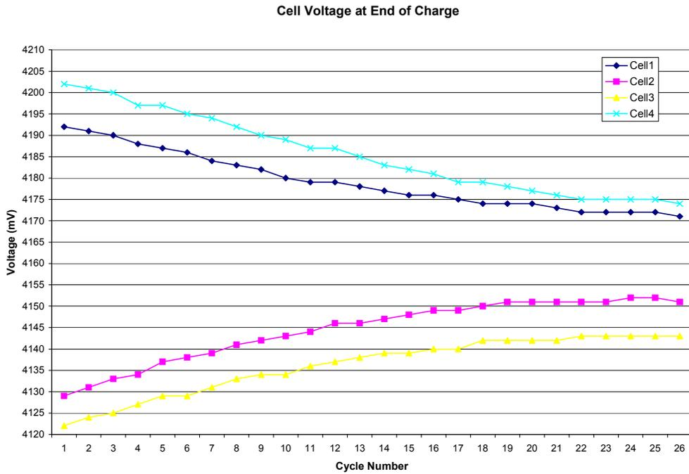
**Figure 8. End-of-Charge Cell Voltages After 1000-Second Rest Period**
