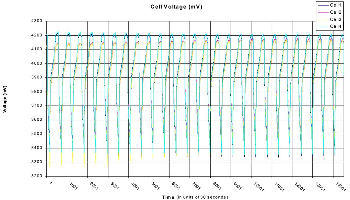
Figure 7. Cell Voltage Over Complete Balancing Cycle
