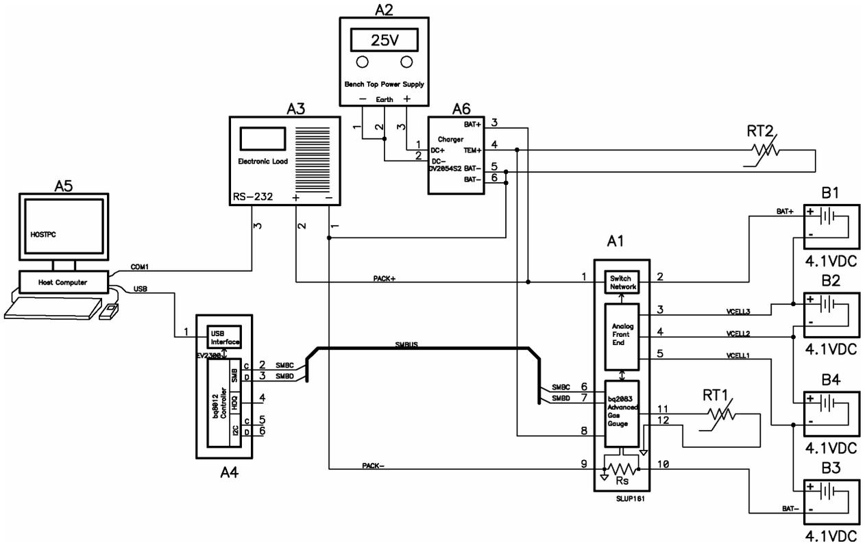
**Figure 4. Hardware Setup for Automatic Cell-Balance Cycling**
