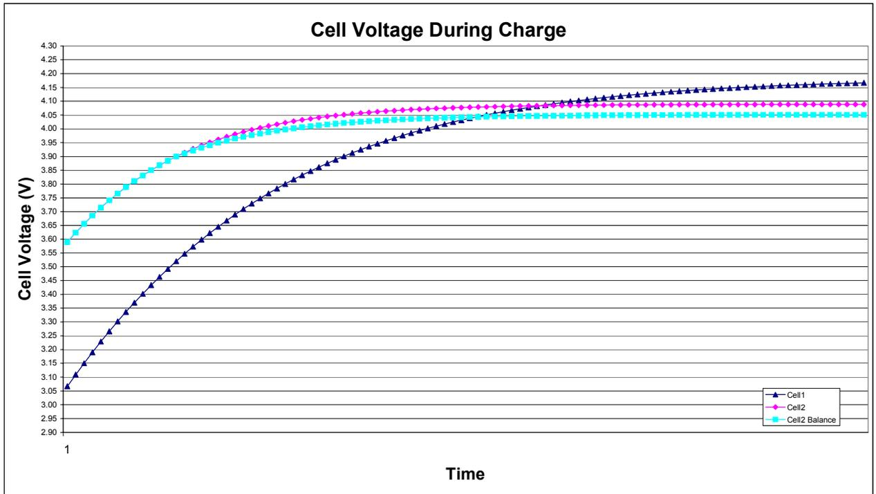
Figure 11. Cell Voltage During Charge, Improper Thresholds
