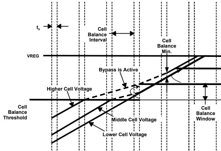
Figure 2. Cell-Balancing Operation
