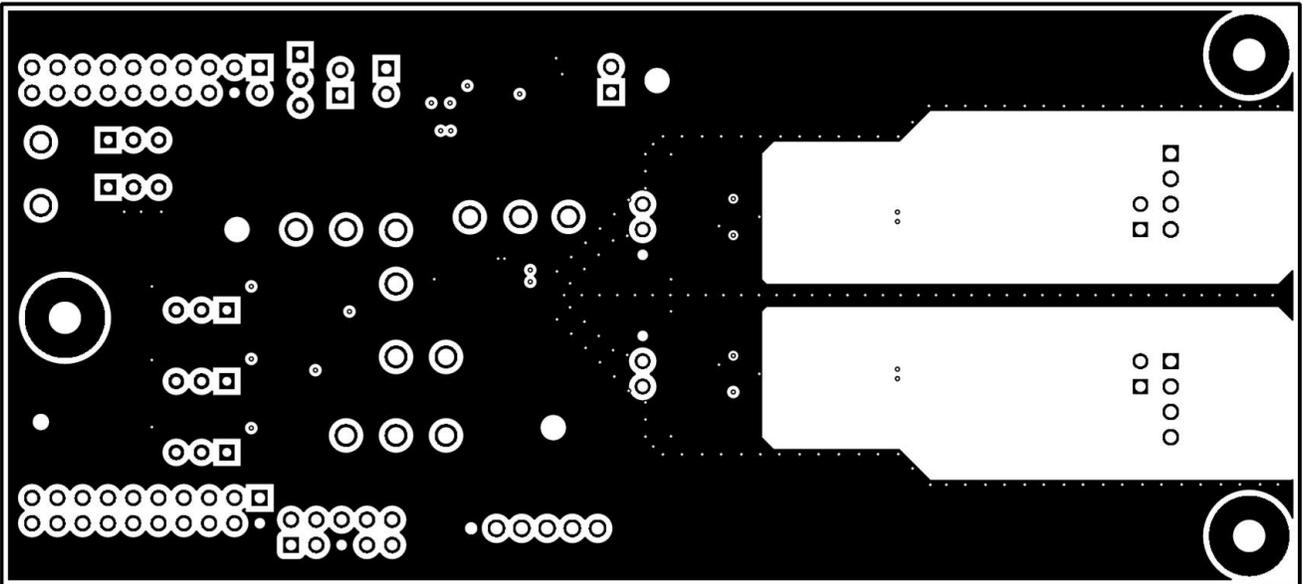
Figure 6-9. BQ79600EVM Internal Signal Layer 1 - GND Plane
