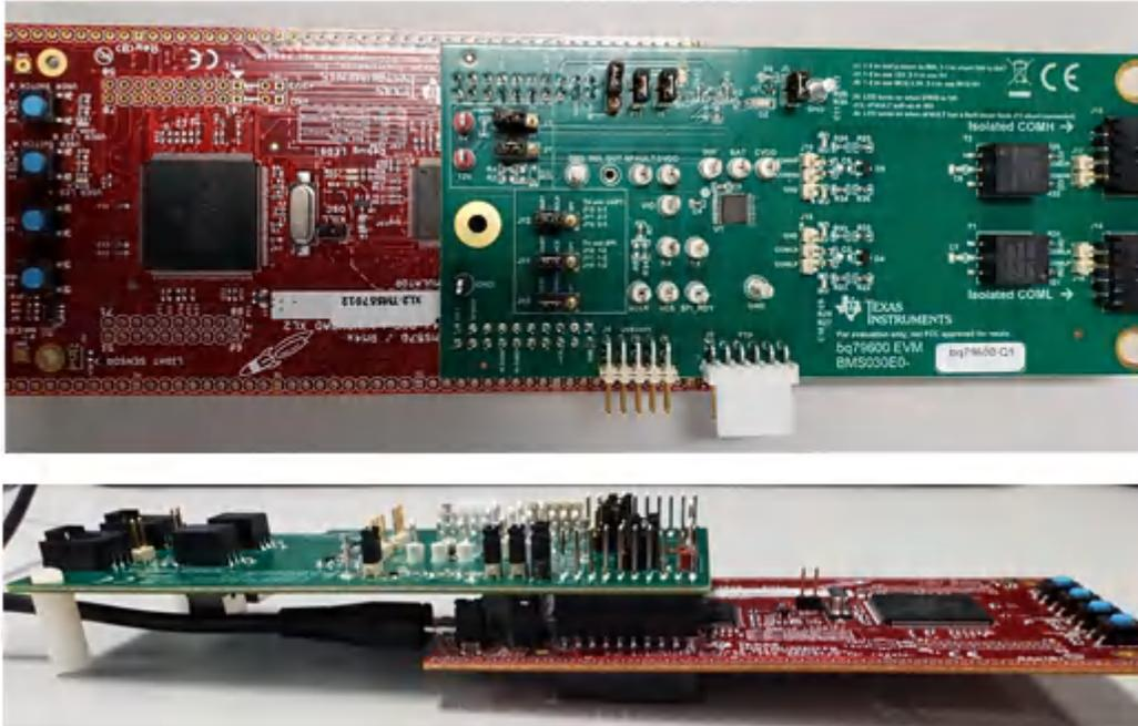
**Figure 4-2. Connection Between BQ79600EVM and TMS570 LaunchPad**
