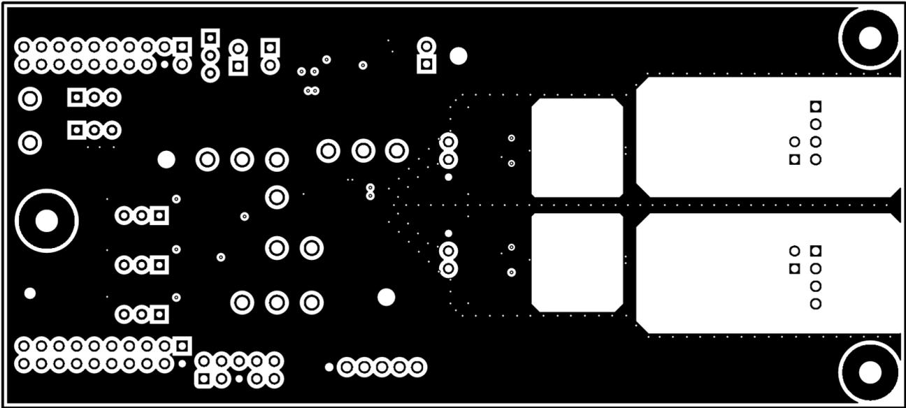
Figure 6-10. BQ79600EVM Internal Signal Layer 2 - GND Plane
