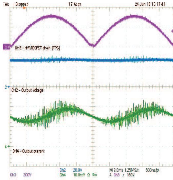
Figure 10. Output Ripple (CH4 – 200 mA/10 mV)
