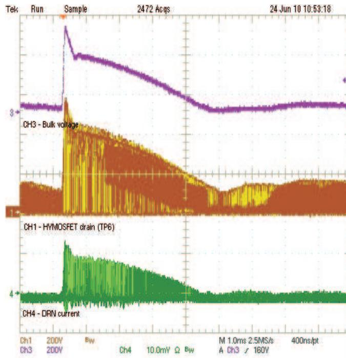
Figure 15. TRIAC Triggering at 50% (CH4 – 500 mA/10 mV)
