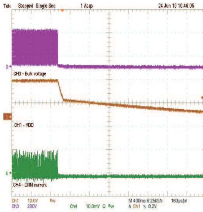
Figure 13. Turn-Off Waveform (CH4 – 500 mA/10 mV)
