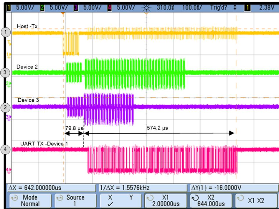
**Figure 18. Test Results for Broadcast Reading Command**
