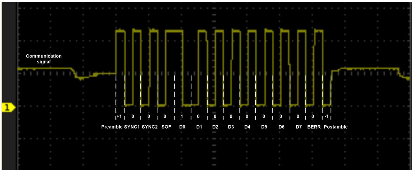
Figure 4. Example Scope Plot of a Byte Structure
