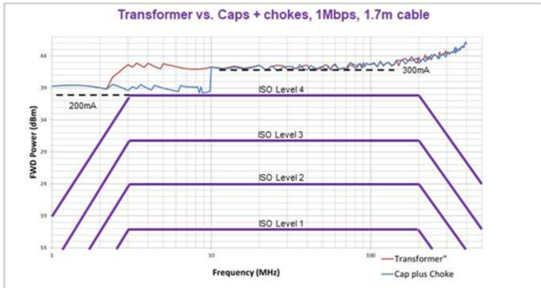
Figure 31. Transformer vs Cap & Choke BCI Plot
