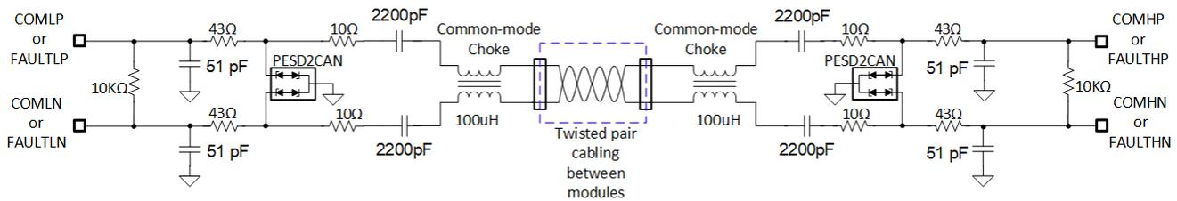
Figure 32. Cap & Choke Isolation Schematic
