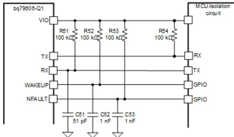
Figure 18. Connecting WAKEUP and Communication for Bottom Device
