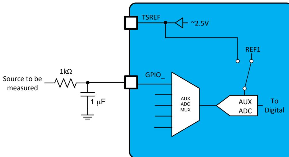
**Figure 12. GPIO Absolute Voltage Measurement**
