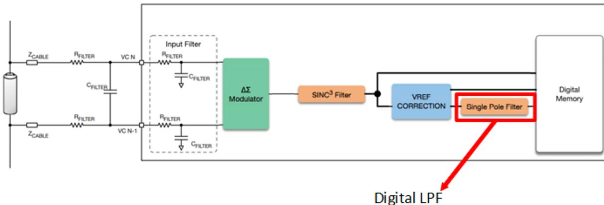
Figure 26. Battery Voltage Signal Chain
