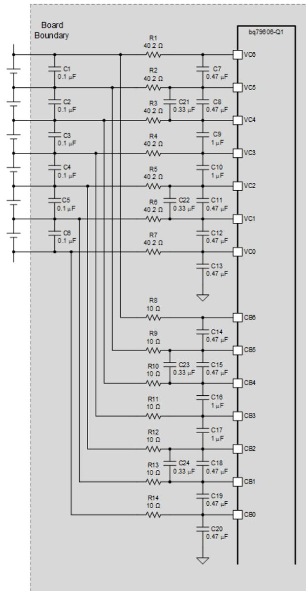
**Figure 9. Cell Voltage Sense and Cell Balancing**
