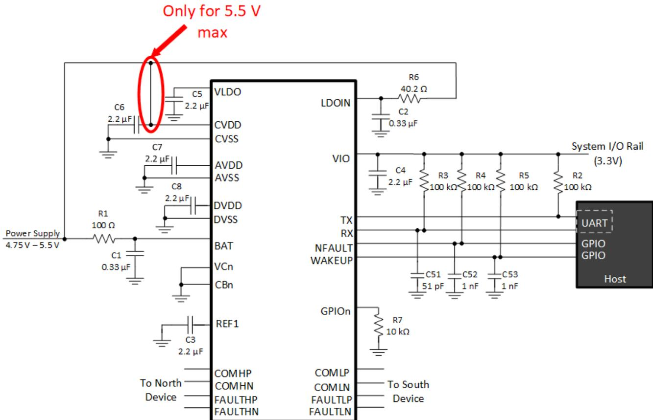
Figure 17. Bridge Device Schematic for 4.75 V to 5.5 V
