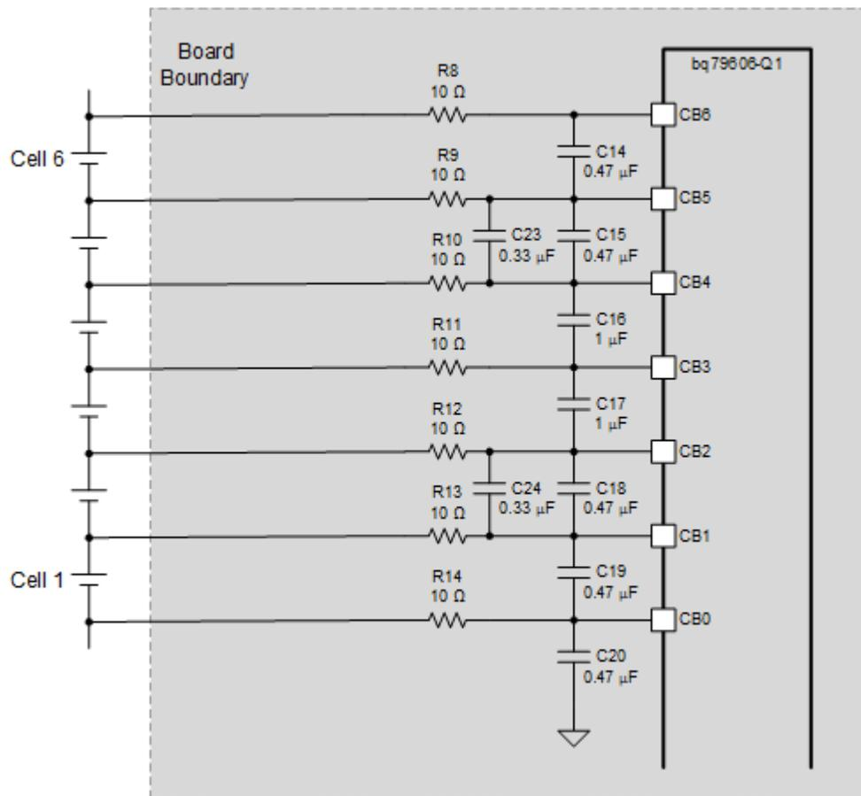
Figure 6. Cell Balancing
