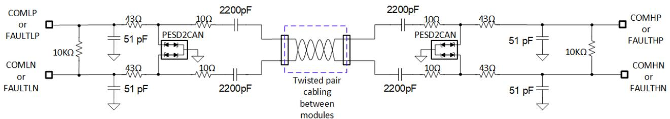
Figure 30. Capacitive Only Isolation Schematic
