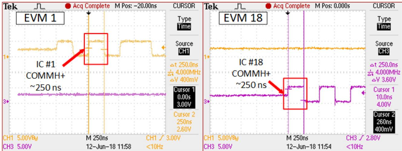
Figure 23. Re-Clocking Bit Compression Example
