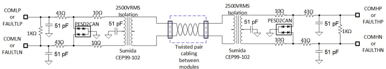
Figure 33. Transformer Isolation Schematic
