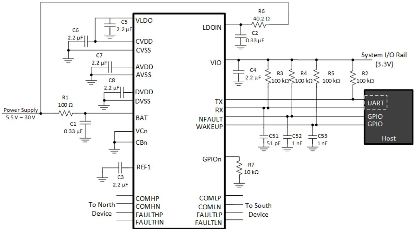
Figure 16. Bridge Device Schematic for 5.5 V - 33 V
