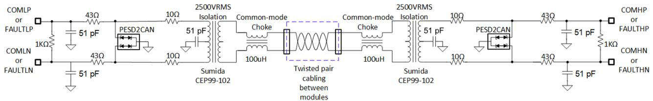
B. Components Required for Transformer Coupled Daisy Chain with Cabling > 2m
