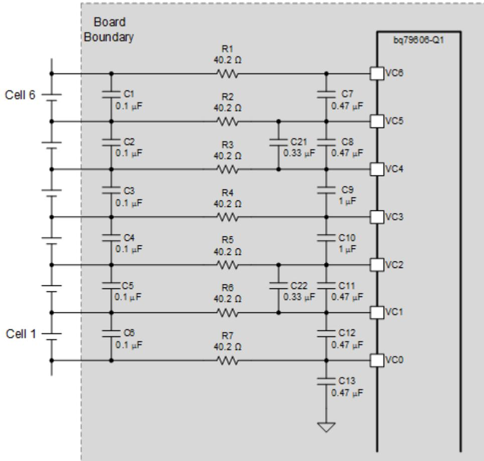
**Figure 5. Cell Voltage Monitoring**
