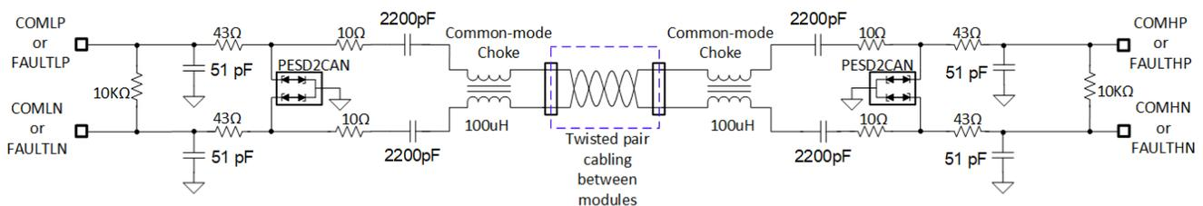
B. Components Required for Capacitive Coupled Daisy Chain with Cabling > 2m
