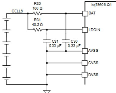
**Figure 1. Power Supply Schematic**
