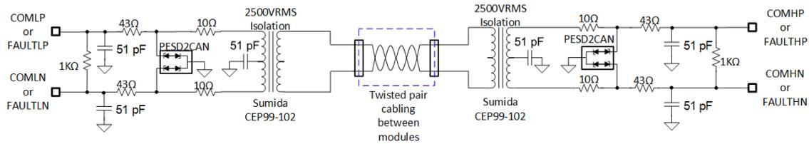
A. Components Required for Transformer Coupled Daisy Chain with Cabling < 2m
