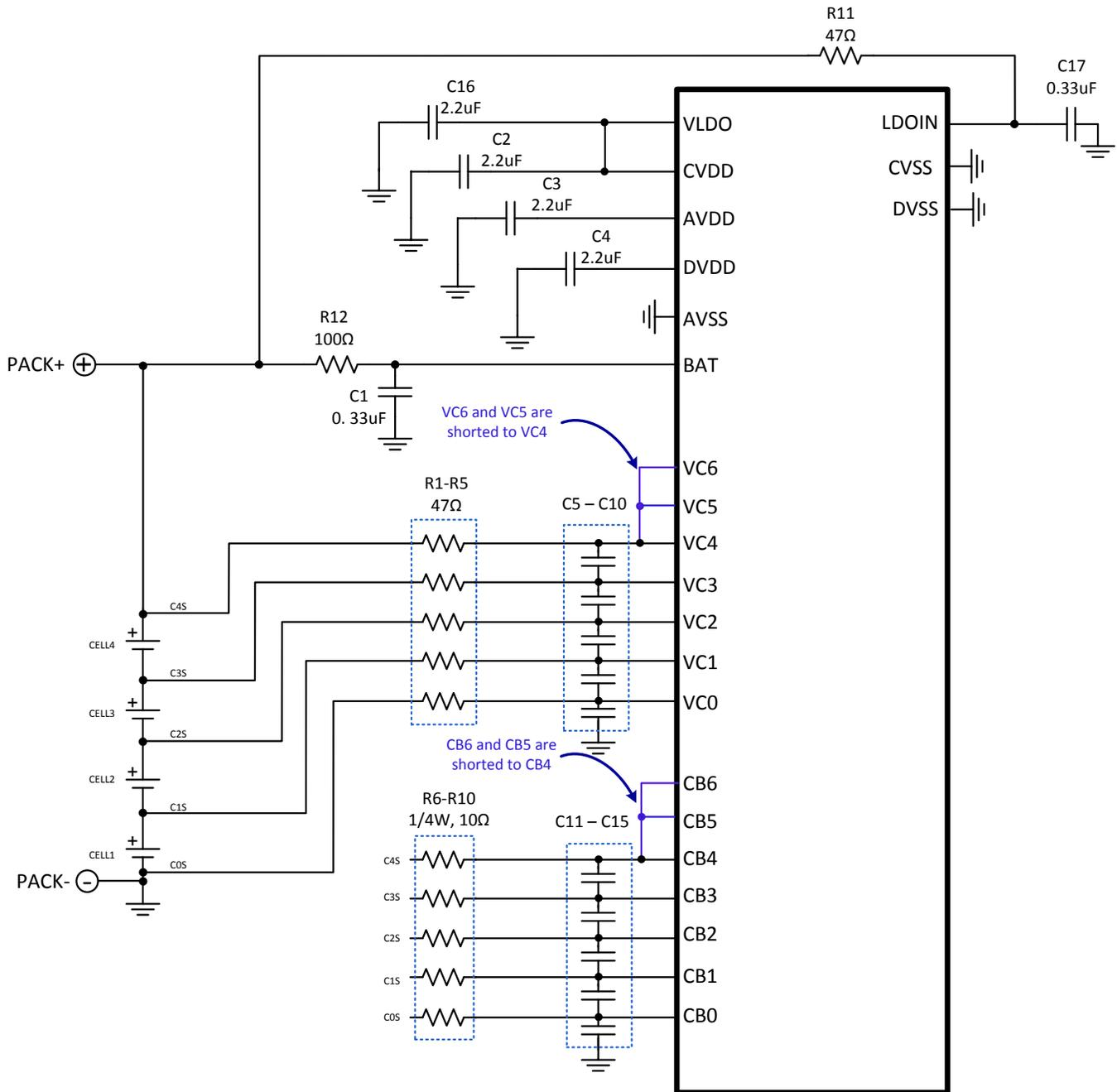
Figure 10. Connecting Fewer than 6 Cells
