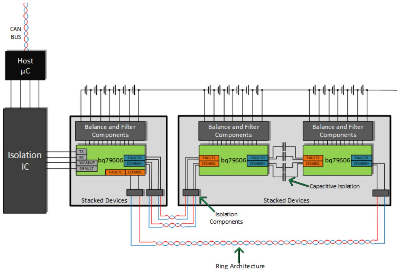
**Figure 15. Using BQ79606A-Q1 with an Isolation Circuit Block Diagram**
