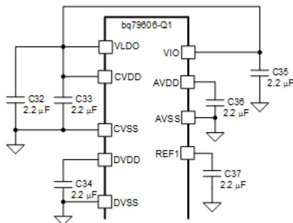
**Figure 3. Regulator Connection for Stack Device**
