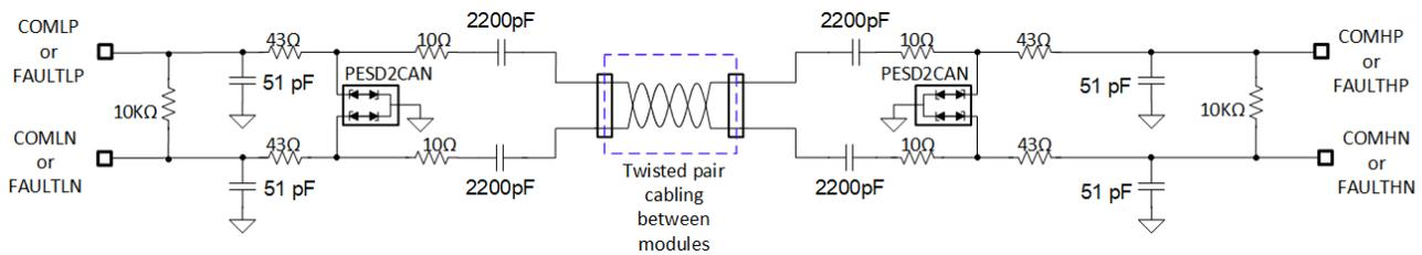
A. Components Required for Capacitive Coupled Daisy Chain with Cabling < 2m
