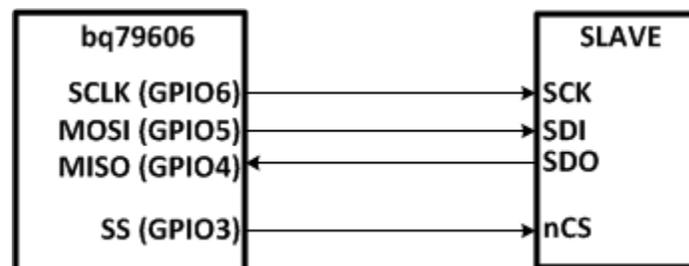
**Figure 13. Example SPI Master Connections**
