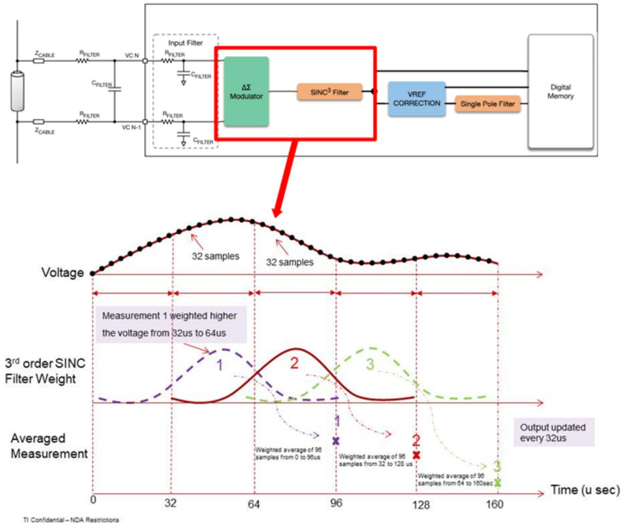
Figure 25. Simplified Signal and Weighting of SINC<sup>3</sup> Filter with DR = 32
