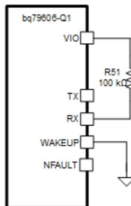
Figure 19. Connecting WAKEUP and Communication for Stacked Device
