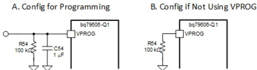
Figure 4. VPROG connection for OTP Programming
