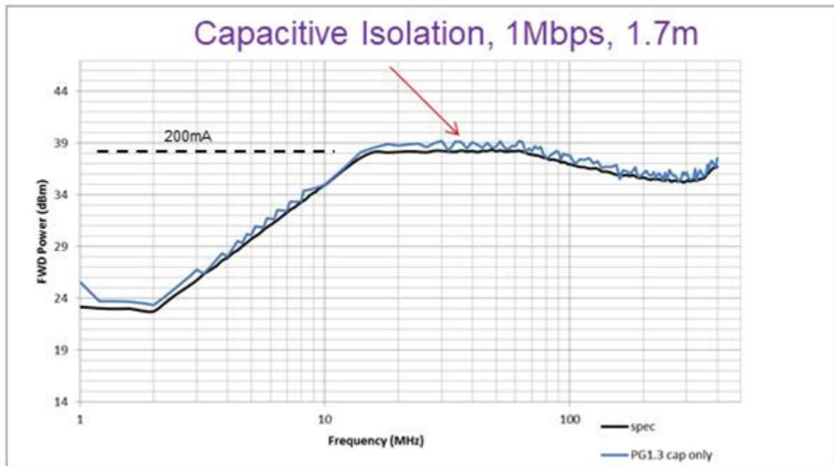
Figure 29. Capacitive Isolation BCI Plot
