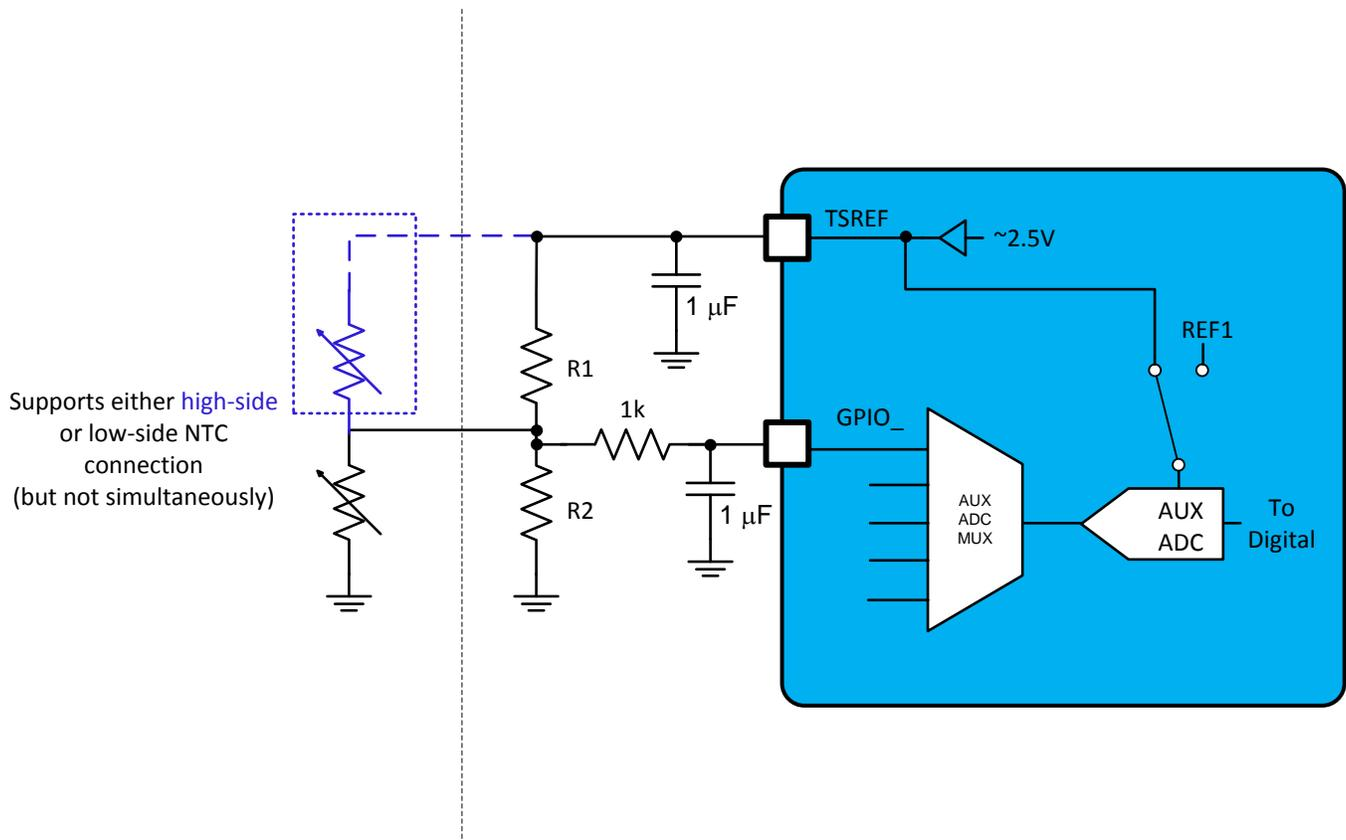
**Figure 11. GPIO Ratiometric Measurement**
