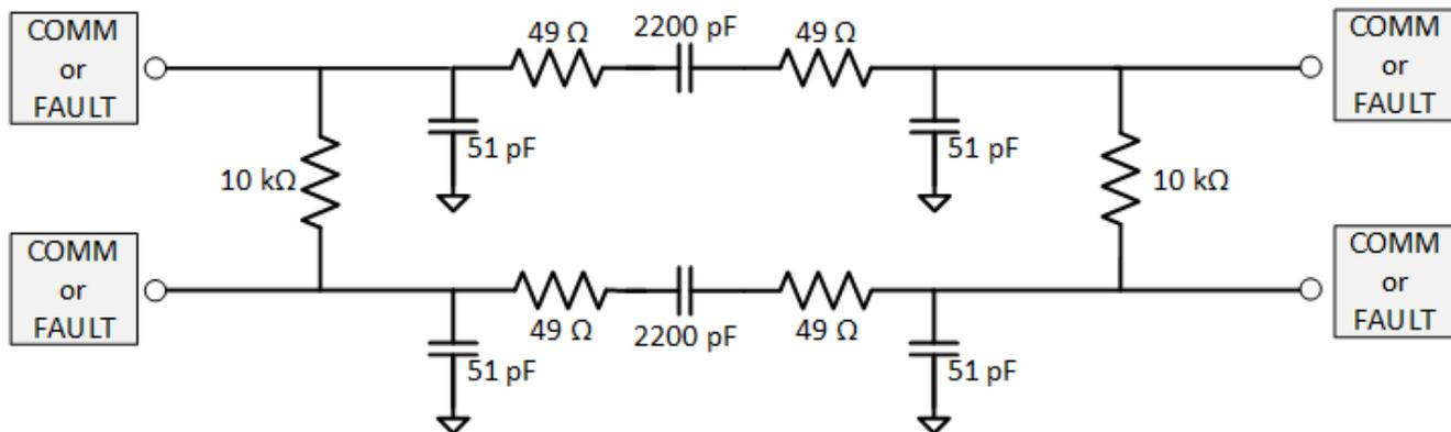
**Figure 20. Noise Isolation for Devices on Same PCB**
