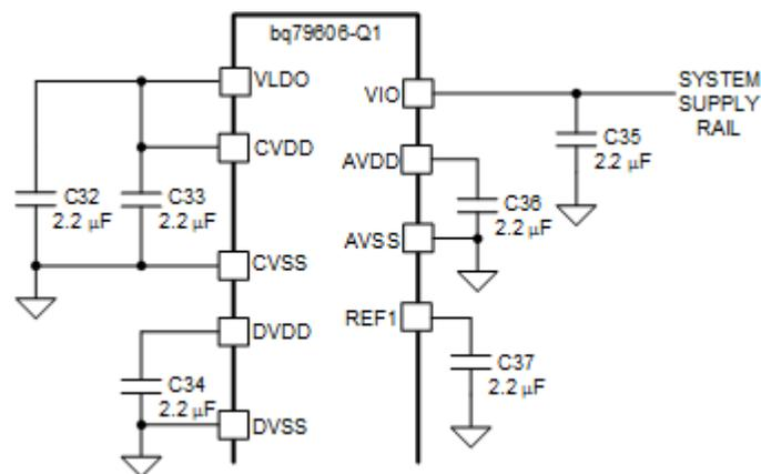
**Figure 2. Regulator Connection for Base Device**
