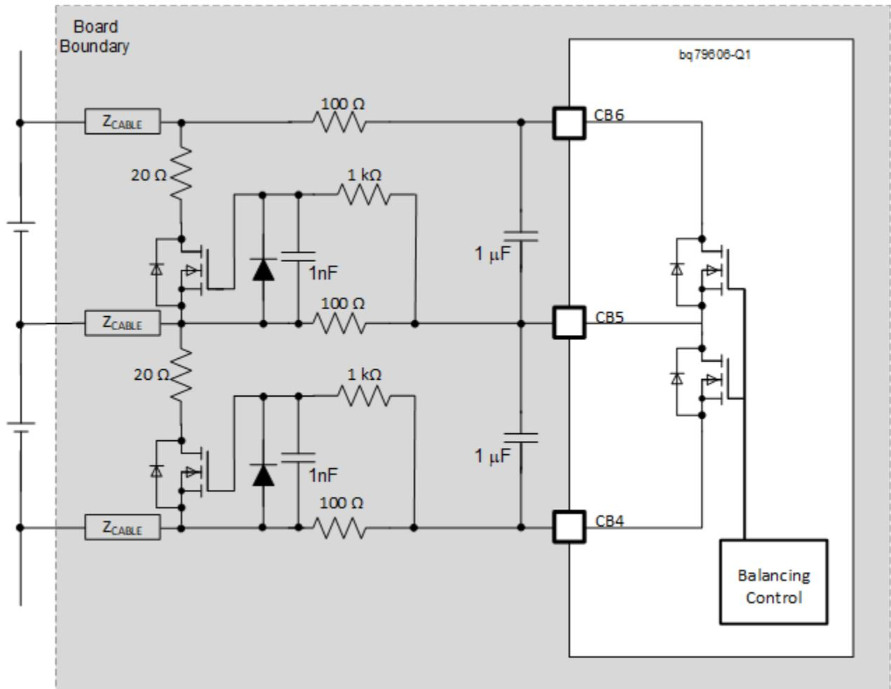
Figure 8. External FET Cell Balancing
