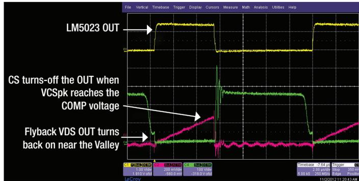
Figure 2. Typical QR switching waveforms
