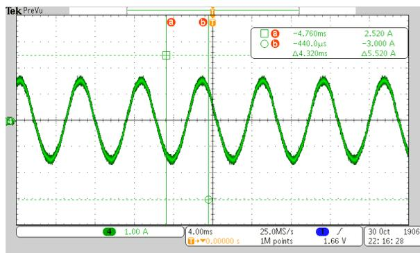
Figure 2-9. MCF8316 Current Waveform in Test 2 Configuration
