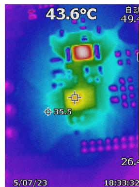
Figure 2-8. MCF8316 Thermal Image in test 1 configuration
