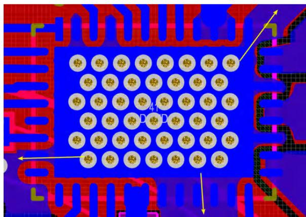
Figure 2-13. MCF831X Heat Dissipation Path (Bottom Layer)
