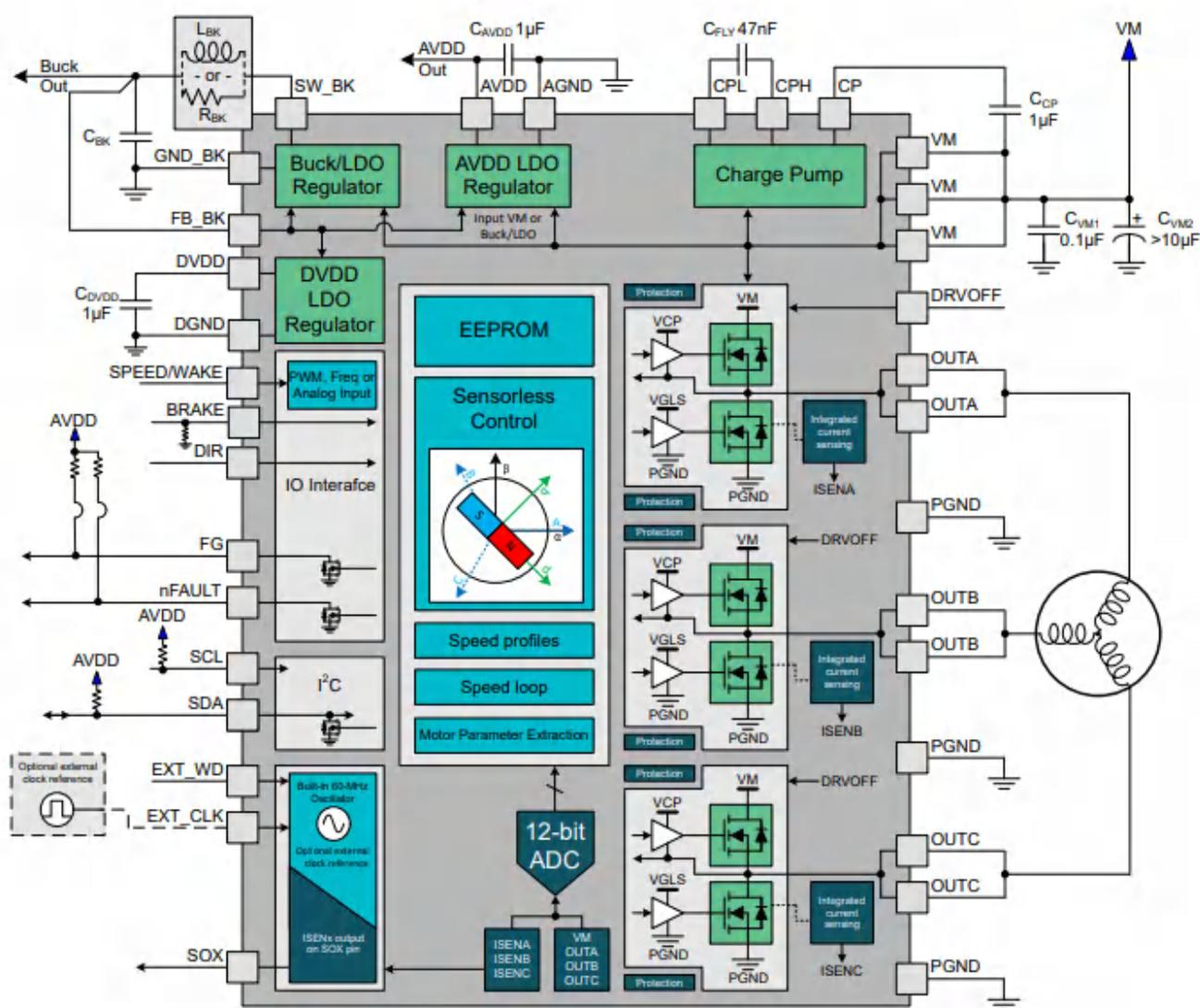
Figure 1-1. MCF831X Block Diagram
