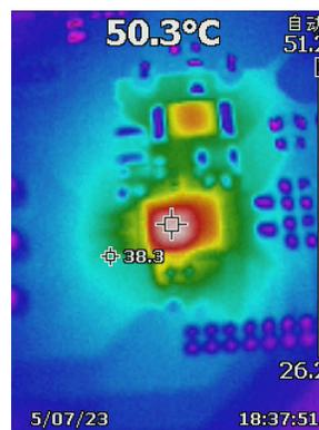
Figure 2-10. MCF8316 Thermal Image in Test 2 Configuration
