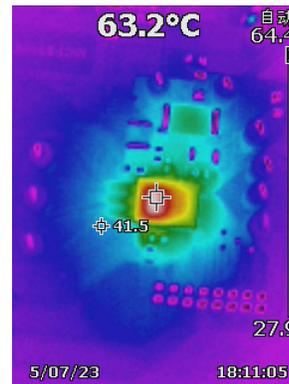
Figure 2-6. MCF8315 Thermal Image in Test 2 Configuration
