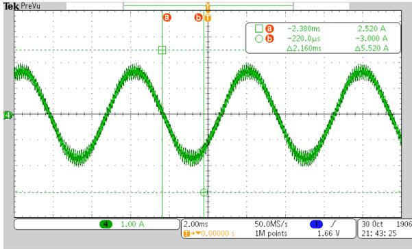
Figure 2-3. MCF8315 Current Waveform in Test 1 Configuration
