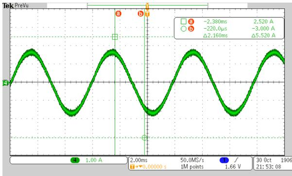
Figure 2-5. MCF8315 Current Waveform in Test 2 Configuration
