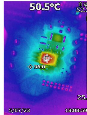
Figure 2-4. MCF8315 Thermal Image in Test 1 Configuration
