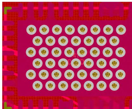
Figure 2-14. MCF831X Heat Dissipation Path (Top Layer)
