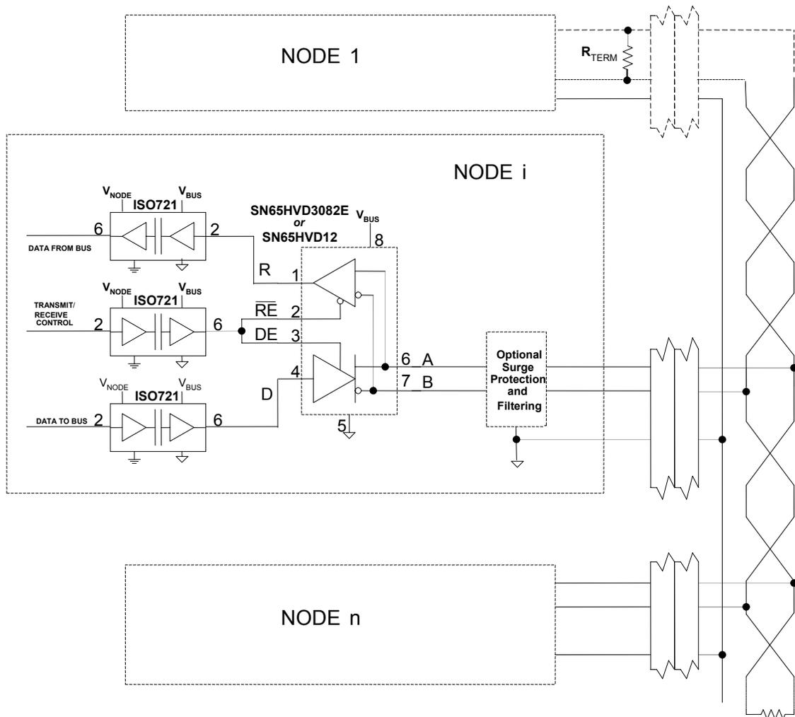
**Figure 2. Typical Isolated RS-485 Circuit Using Digital Isolators**
