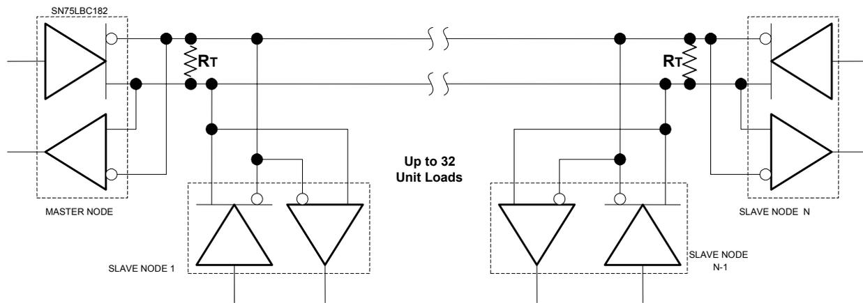
**Figure 1. Half-Duplex 485 Network With Single Master and Multiple Slave Nodes**
