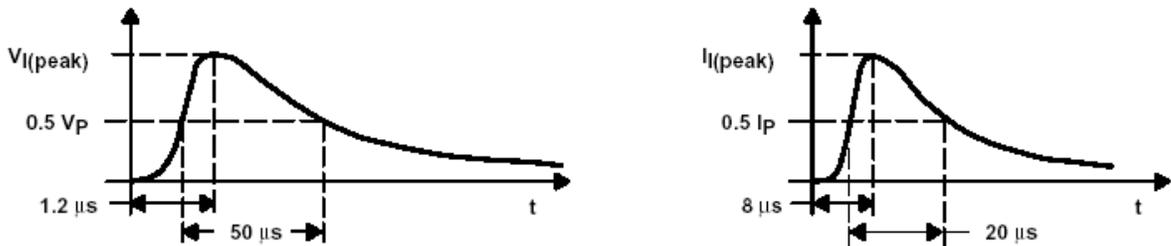
**Figure 5. Waveforms for Transient Voltage testing**
