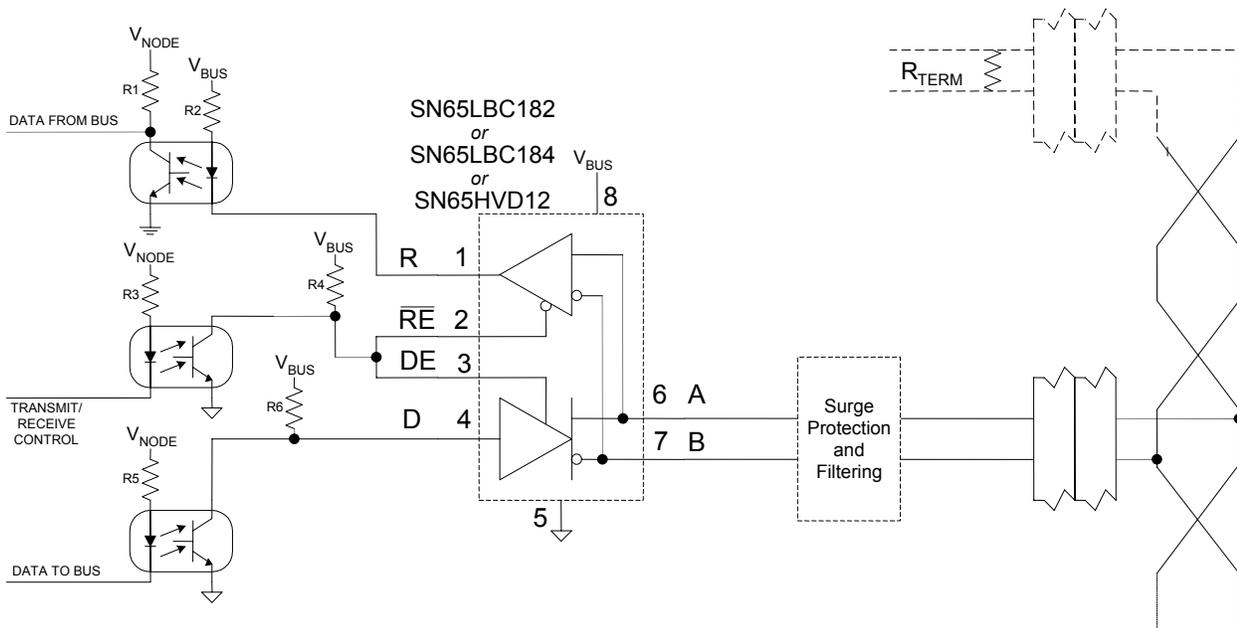
**Figure 3. Typical Isolated RS-485 Interface Circuit Using Optocouplers**
