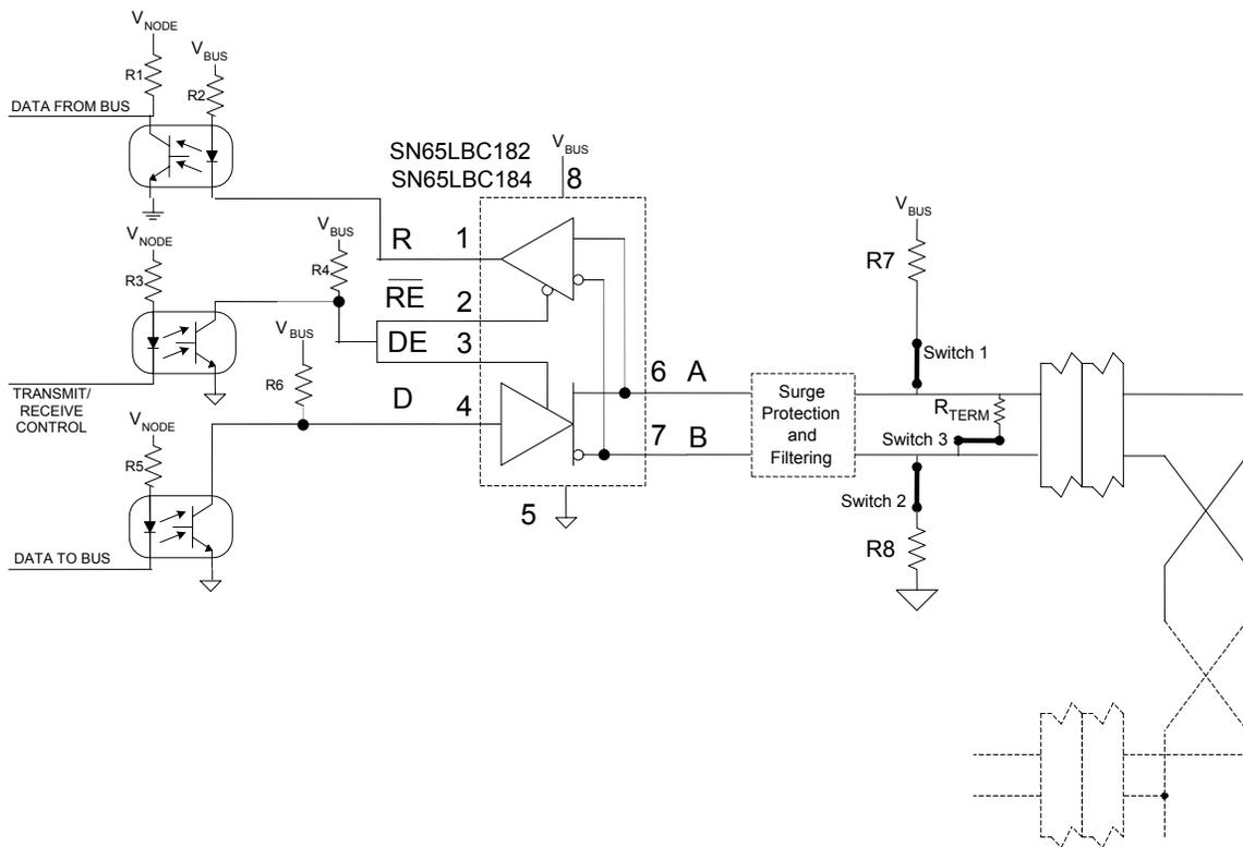
**Figure 4. Typical Terminal Node With Termination and Failsafe Biasing Resistors**
