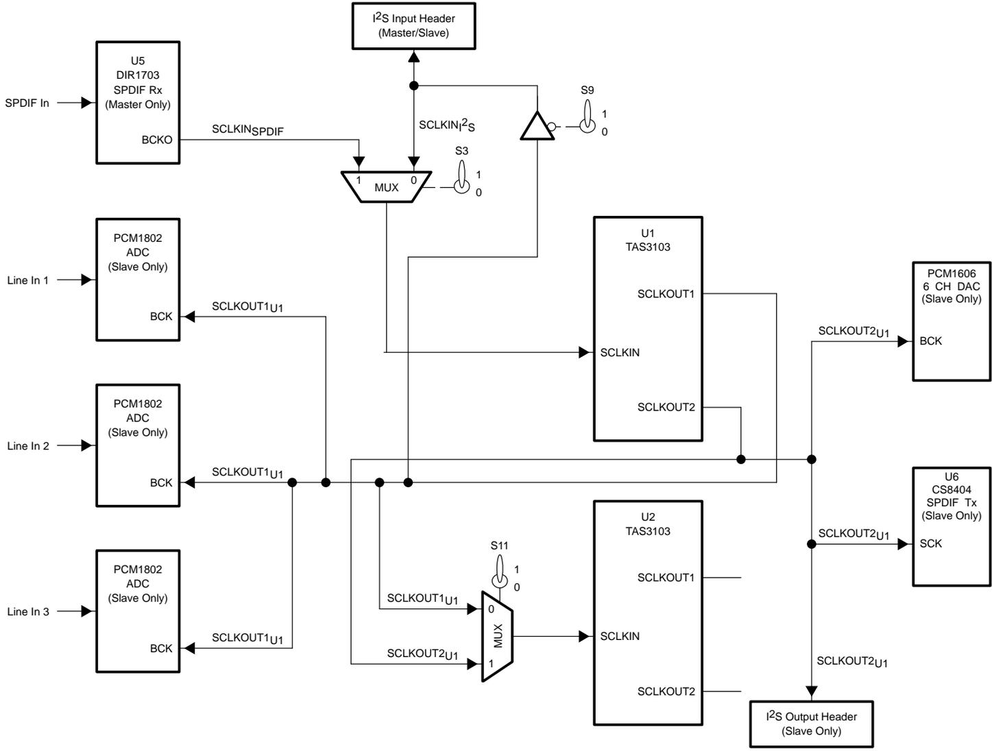
SCLKOUT1 of TAS3103–U1 serves as the SCLK for the ADCs and SCLKOUT2 of TAS3103–U1 serves as the SCLK for the 6-channel DAC and the SPDIF Tx. Both SCLKOUT clocks are routed to a multiplexer. Switch S11 selects whether SCLKOUT1 of TAS3103–U1 (S11 set to L) or SCLKOUT2 of TAS3103–U1 (S11 set to H) is routed to pin SCLKIN of TAS3103–U2. This multiplexer is necessary as either clock can be the higher frequency clock in certain applications and SCLKIN must be provided the higher of the two clocks.
