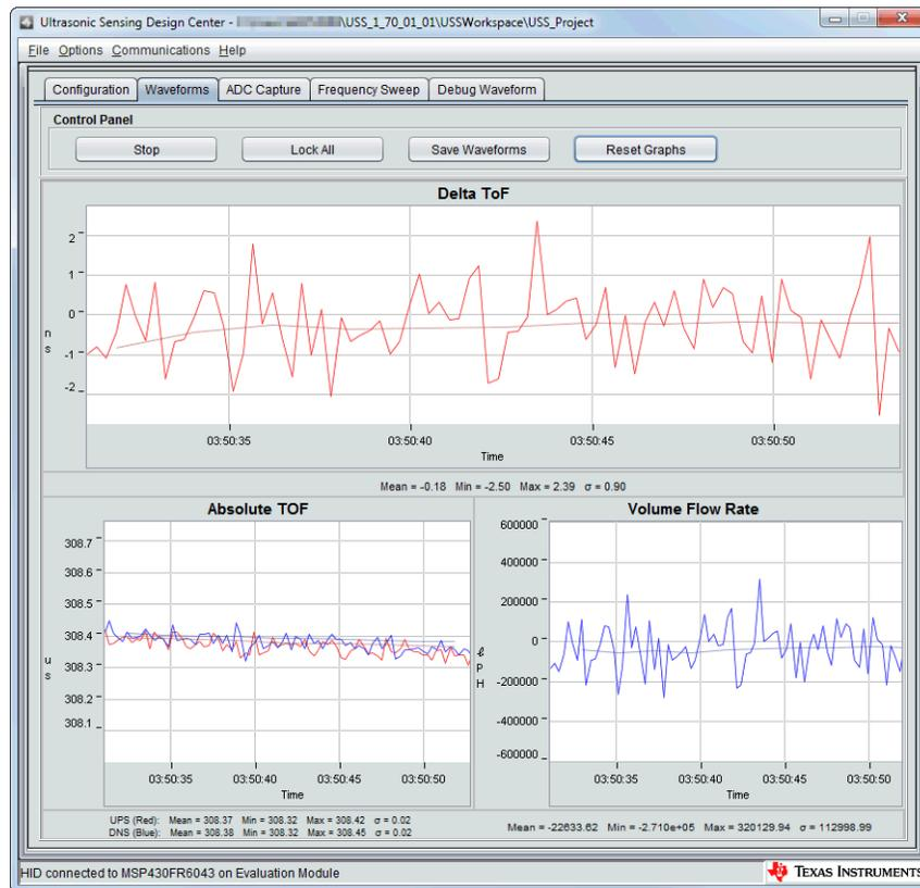
**Figure 7. Waveforms in Design Center**
