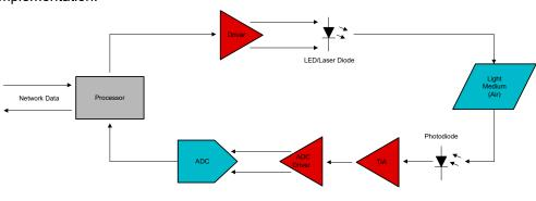
Figure 1. LiFi Signal Chain Block Diagram
