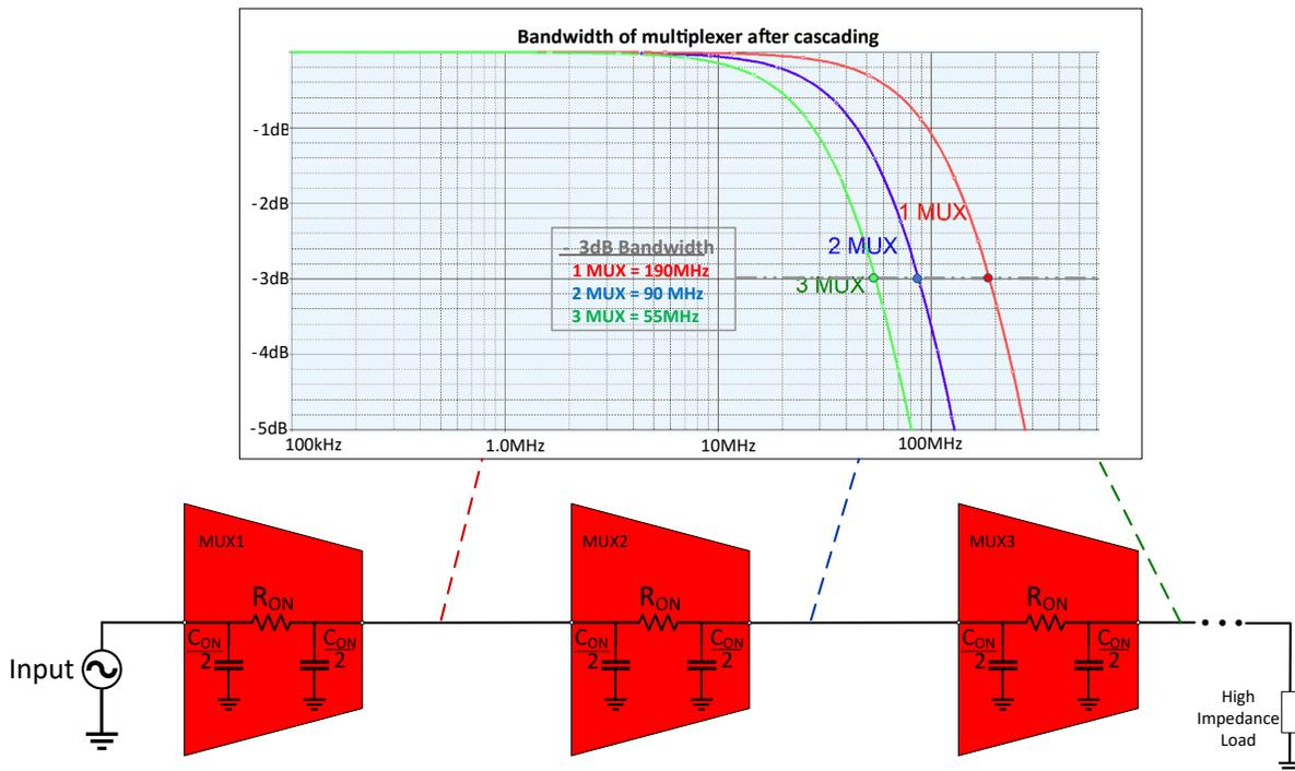
Figure 2-6. On-Resistance Effects on -3dB Bandwidth (High Impedance Load)
