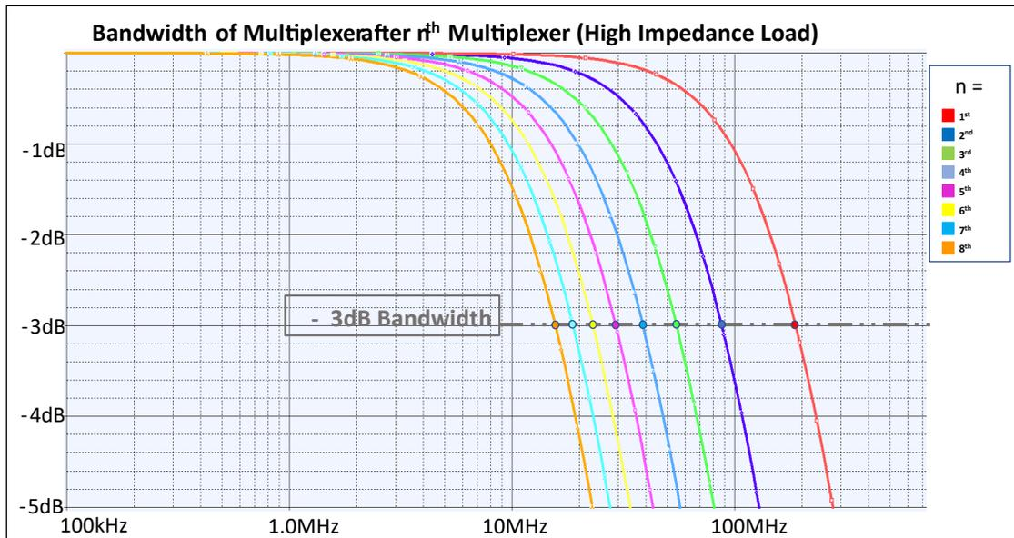
Figure 2-7. -3dB Bandwidth of  $n^{\text{th}}$  Multiplexer (High Impedance Load)
