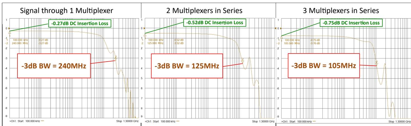
**Figure 2-9. Experimental Results of 3 Multiplexers in Series**
