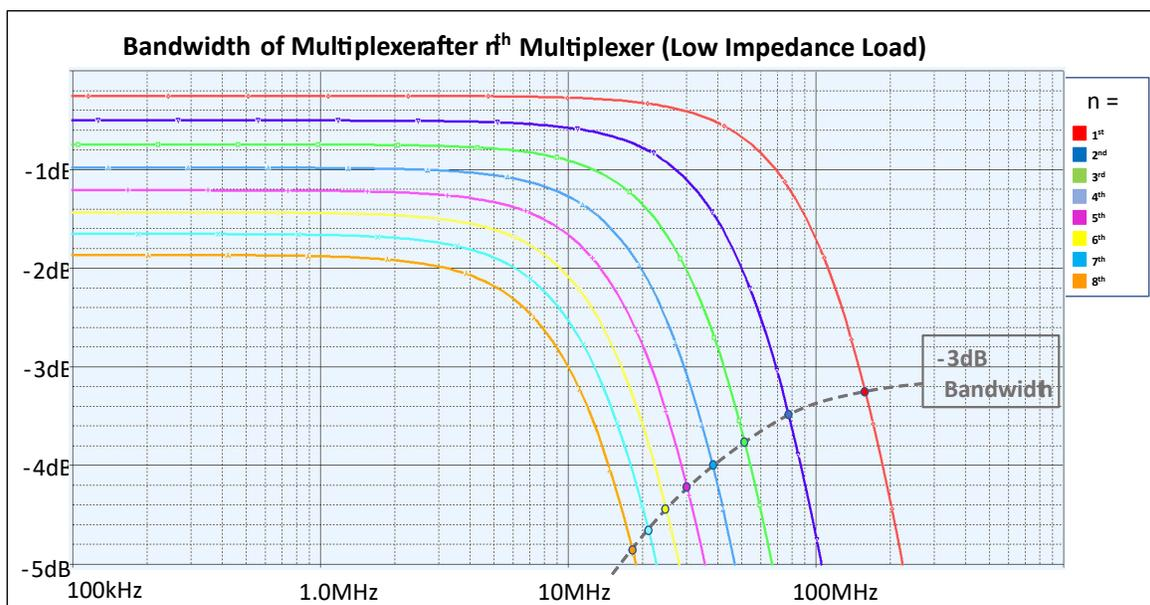
Figure 2-8. -3dB Bandwidth of  $n^{\text{th}}$  Multiplexer (Low Impedance Load)
