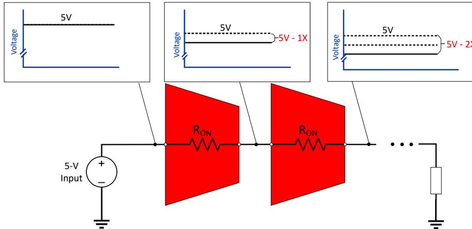
Figure 2-1. Effects of On-Resistance when Cascading Multiplexers
