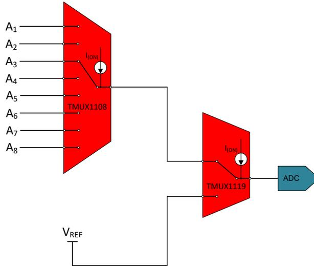
Figure 2-3. Cascading Precision Multiplexers
