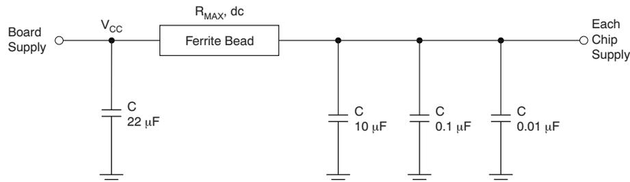
**Figure 18. Power-Supply Decoupling**
