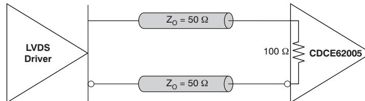
Figure 14. LVDS DC Termination Circuit
