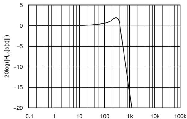
Figure 4. Jitter Peaking Around PLL Bandwidth
