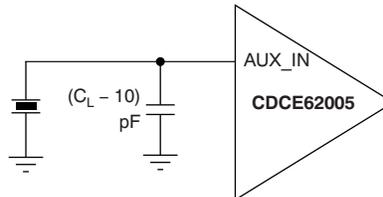
Figure 17. Crystal Input to the CDCE62005
