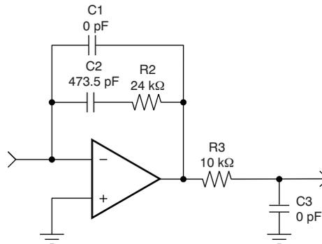
**Figure 5. On-Chip Loop Filter Circuit for Large Loop Bandwidth (>100 kHz)**
