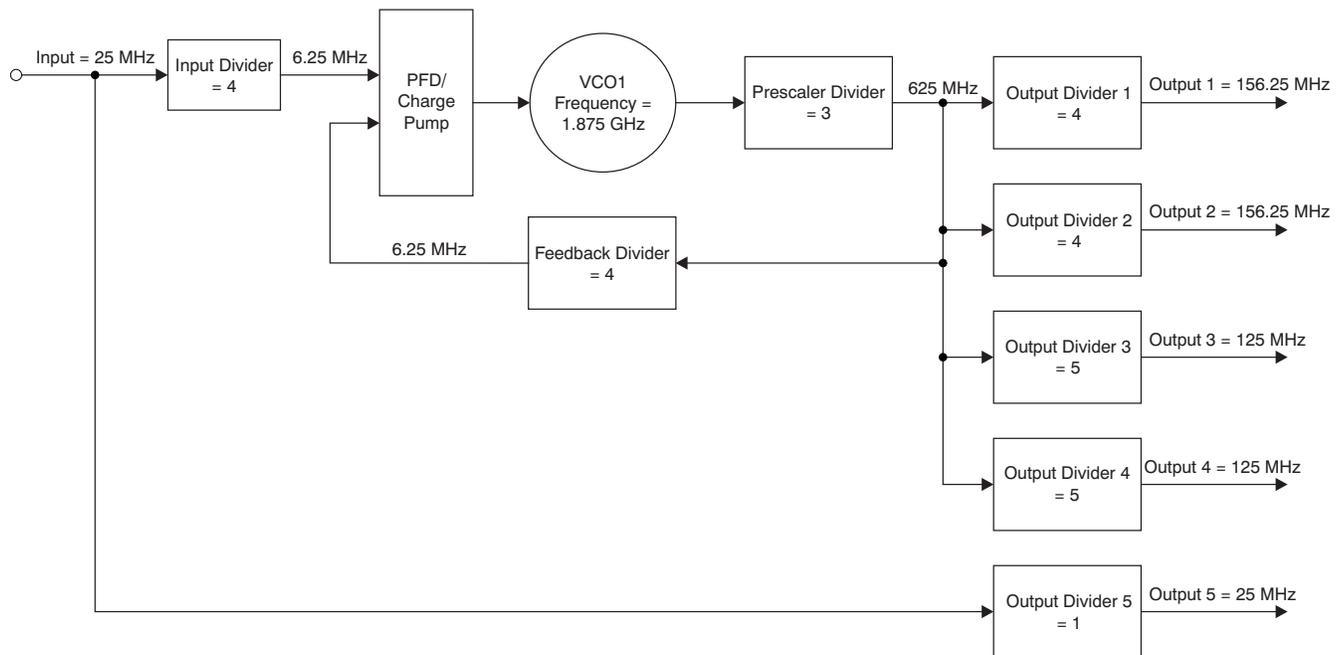
**Figure 2. CDCE62005 Settings for Multiple Frequency Synthesis Example**
