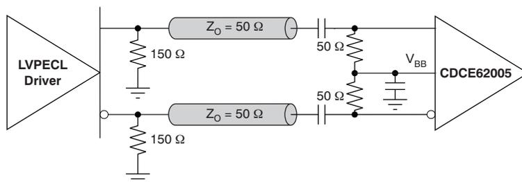
Figure 13. LVPECL AC-Coupled Termination Circuit
