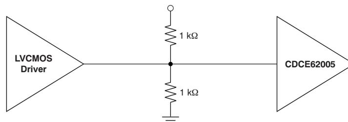
Figure 16. 3.3-V LVCMOS DC-Coupled Termination Circuit
