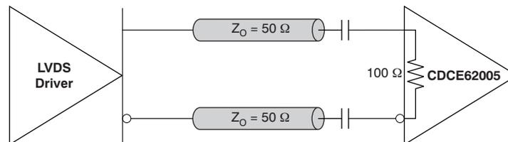
Figure 15. LVDS AC-Coupled Termination Circuit
