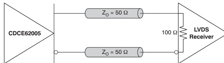
Figure 9. LVDS DC Termination Circuit
