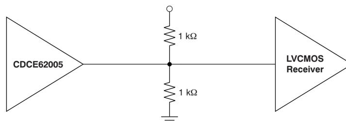
Figure 11. 3.3-V LVCMOS DC-Coupled Termination Circuit
