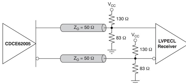
Figure 7. LVPECL DC Termination Circuit
