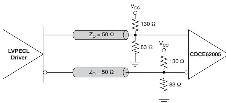
Figure 12. LVPECL DC Termination Circuit
