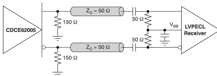
Figure 8. LVPECL AC-Coupled Termination Circuit
