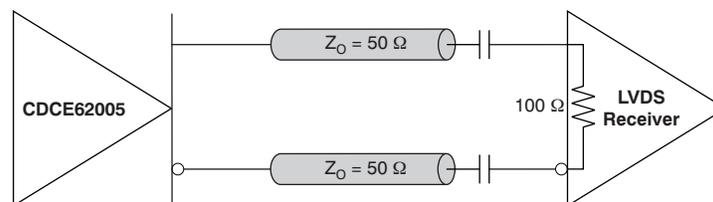
Figure 10. LVDS AC-Coupled Termination Circuit
