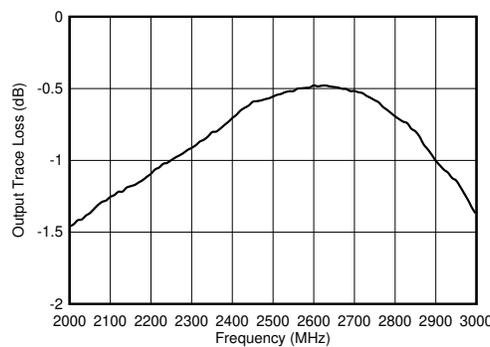
Figure 10. Output PCB Trace Loss vs Frequency
