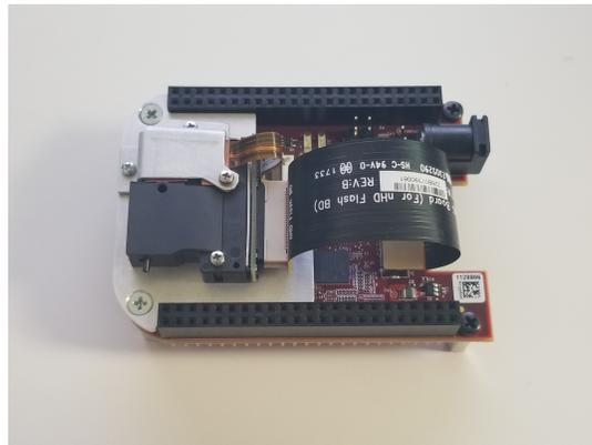
**Figure 1-2. DLP Module 2000 EVM (Installed to DLPDLCR2000EVM, not included with DLPM2000EVM)**
