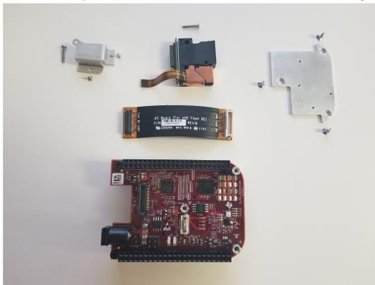
**Figure 2-1. Disassembled EVM Assembly**
