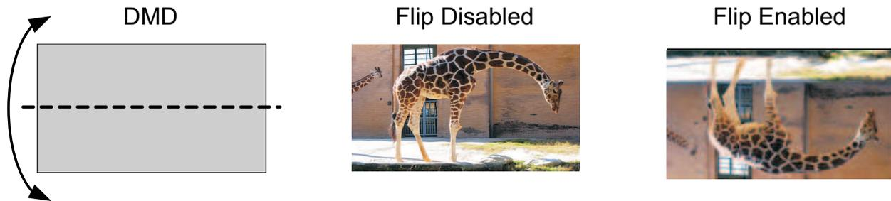
Figure 2-3. Image Short-Axis Flip Example
