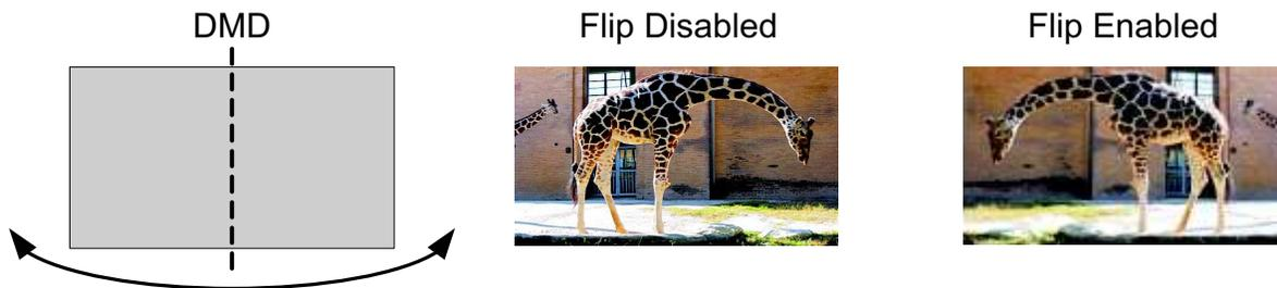
Figure 2-2. Image Long-Axis Flip Example
