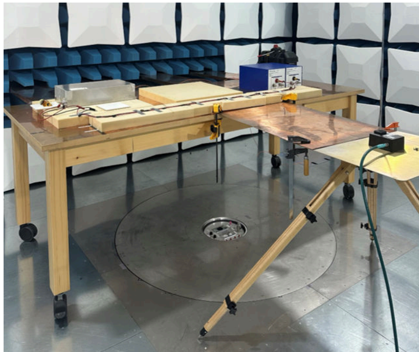
Figure 3-7. CISPR 25 Class 5 Test Setup for the TIDA-060048
