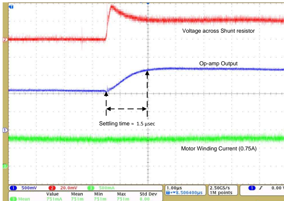
Figure 13. Rising Edge Step Response of Current Sense Amplifier for Positive Current
