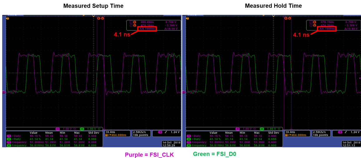
Figure 11. LVDS - FSIRX Setup and Hold Time Measurements
