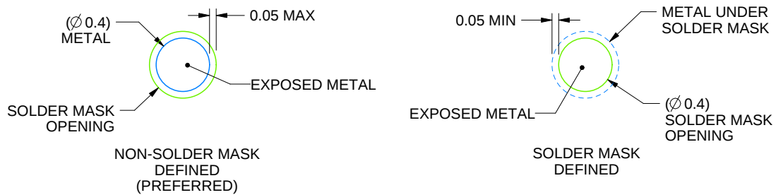
SOLDER MASK DETAILS NOT TO SCALE
