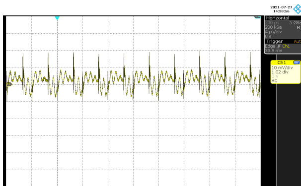
Figure 6-14. Isolated Output V_{O4} Ripple Voltage Under 150-mA Load
