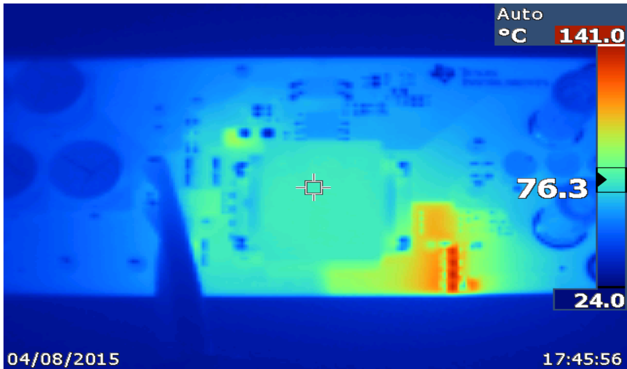
Thermal image was taken at 60Vin, 5A load when the board reaches equilibrium.
