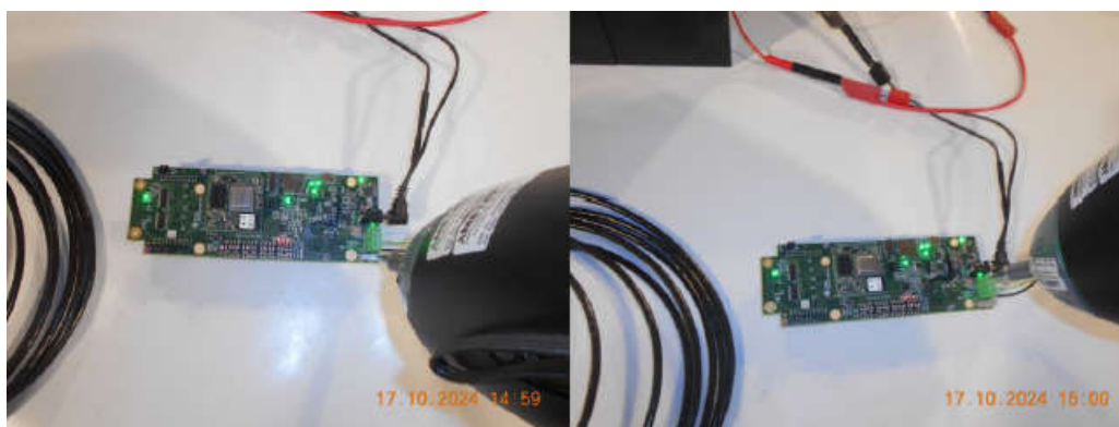
Figure 6-5. ESD Injection on TIDA-010261
