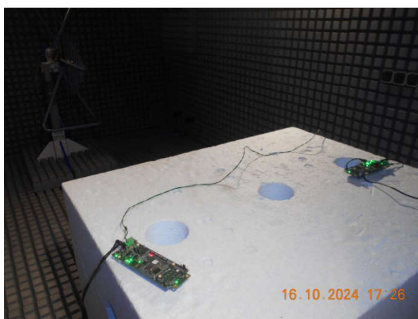
Figure 5-3. Two Connected TIDA-010261 With Single Pair Ethernet
