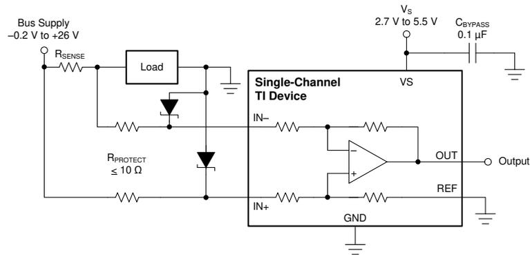
**Figure 8-9. Transient Protection Using Dual Zener Diodes**
