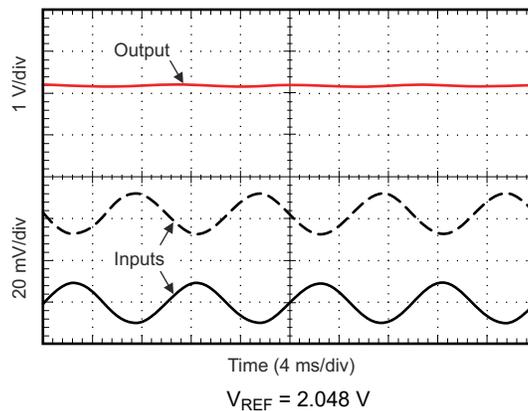
**Figure 8-6. Current Differencing Application Output Response (A2 Devices)**
