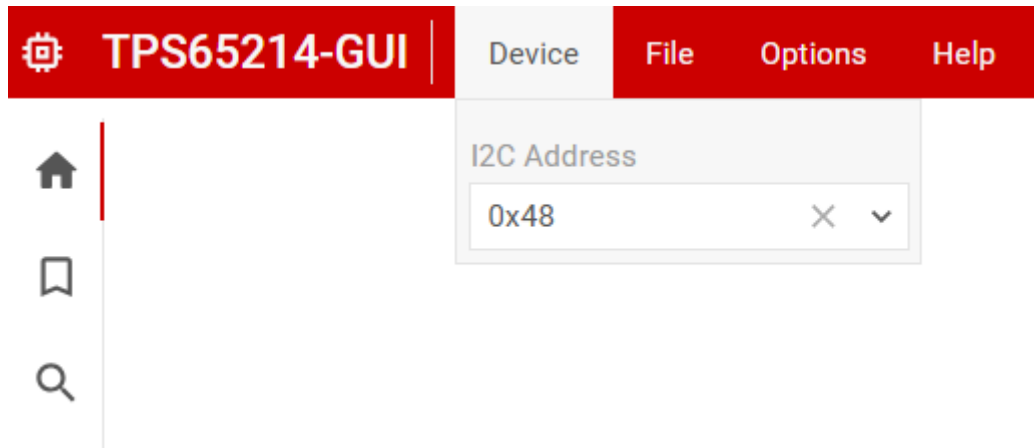
Figure 4-2. Setting I2C address in the GUI
