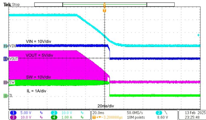
Figure 3-4. TPS561300EVM Shutdown Relative to  $V_{IN}$
