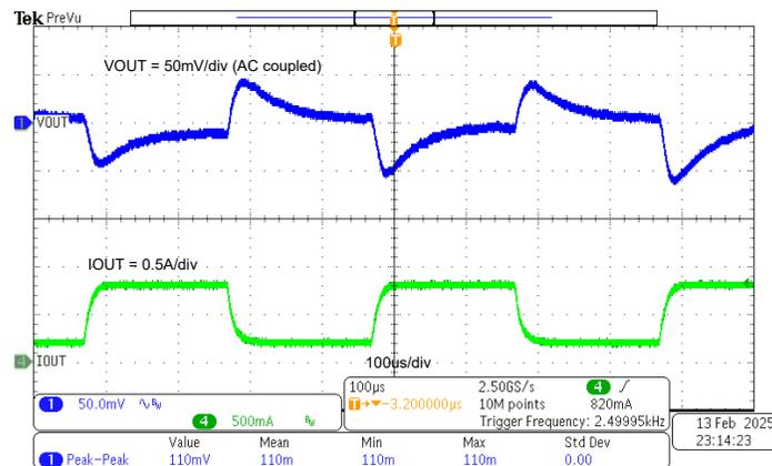
Figure 3-1. TPS561300EVM Load Transient Response, 0.2A to 0.8A Load Step
