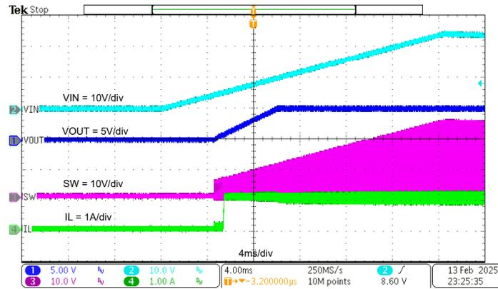
Figure 3-3. TPS561300EVM Start-Up Relative to  $V_{IN}$
