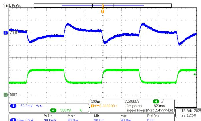
Figure 3-2. TPS561300EVM Load Transient Response, 0.5A to 1A Load Step
