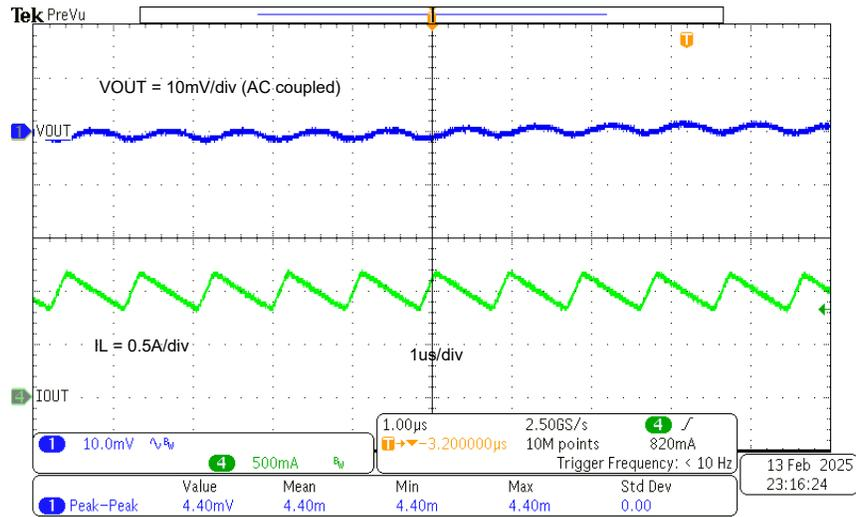
Figure 3-5. TPS561300EVM Output Voltage Ripple,  $I_{OUT} = 1A$
