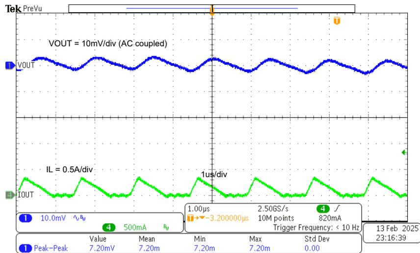
Figure 3-6. TPS561300EVM Output Voltage Ripple,  $I_{OUT} = 0.1A$
