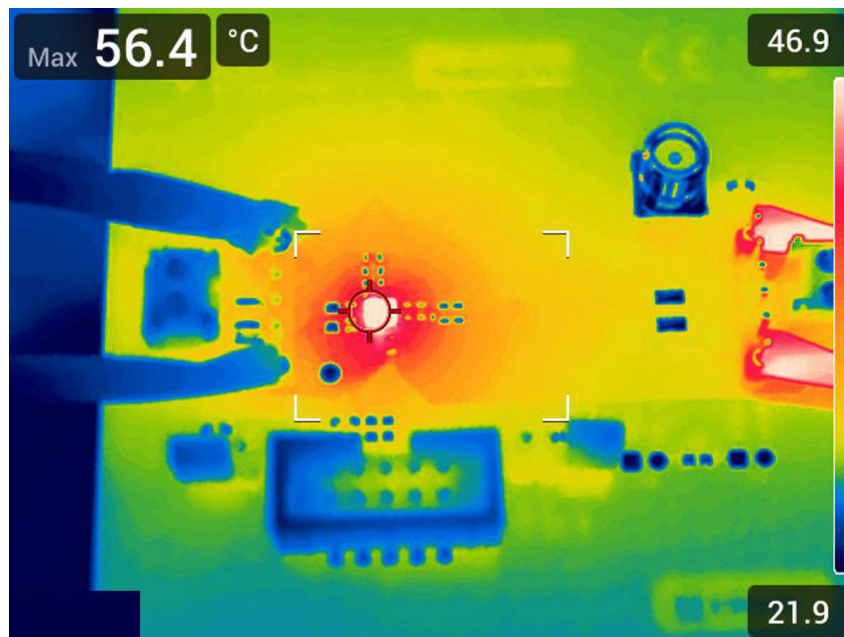
Figure 4-3. Thermal Performance (TPSM82866CA1PEVM, V_{IN} = 5V , V_{OUT} = 0.5V , I_{OUT} = 6A )
