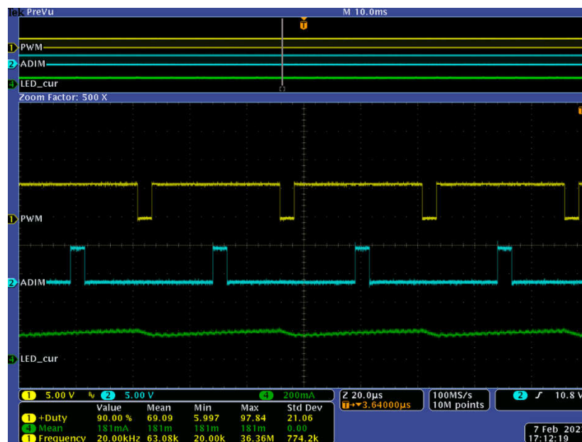
Figure 5-15. Waveforms at 10% Duty Cycle ADIM/HD and 90% Duty Cycle PWM/EN
