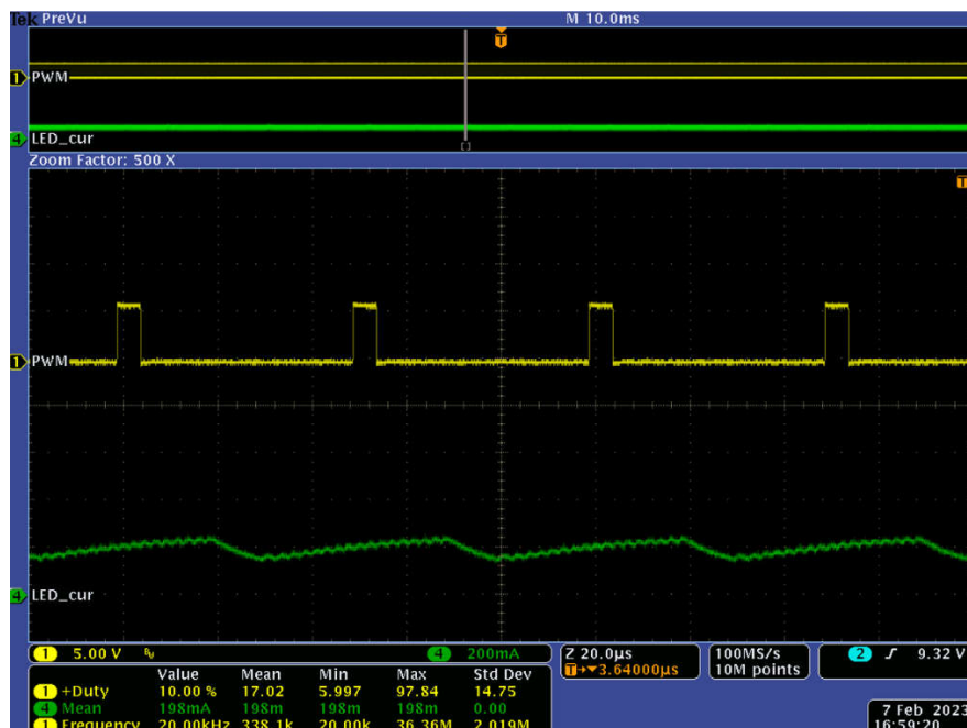
Figure 5-11. Waveforms at 10% Duty Cycle, 20kHz Hybrid Dimming
