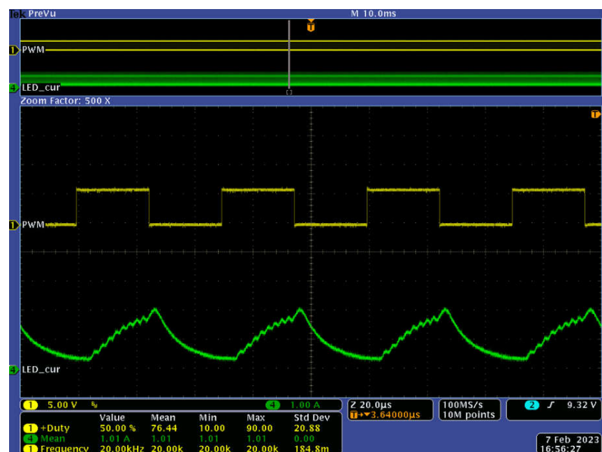
Figure 5-8. Waveforms at 50% Duty Cycle, 20kHz PWM Dimming
