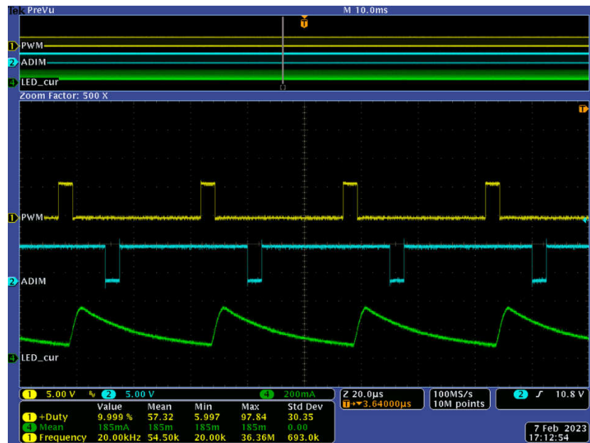
Figure 5-16. Waveforms at 90% Duty Cycle ADIM/HD and 10% Duty Cycle PWM/EN
