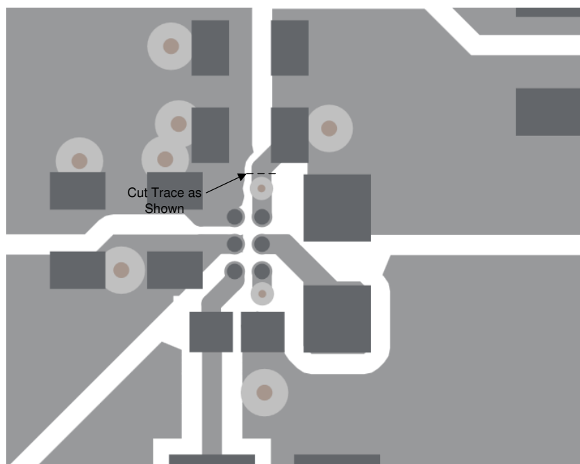
Figure 1-1. Loop Response Measurement Modification
