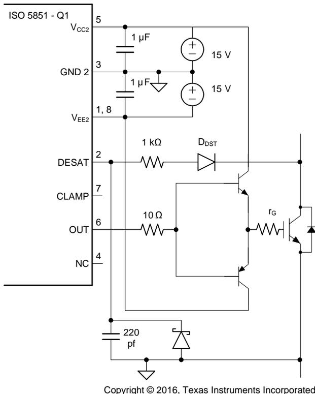
Figure 51. Current Buffer for Increased Drive Current
