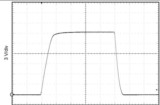
$C_L = 100 \text{ nF}$        $R_G = 0 \Omega$
