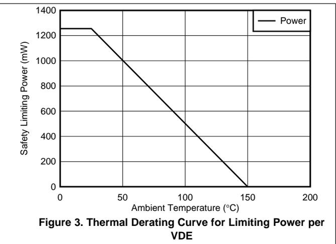
**Figure 3. Thermal Derating Curve for Limiting Power per VDE**
