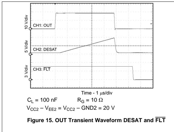
Figure 15. OUT Transient Waveform DESAT and  $\overline{FLT}$
