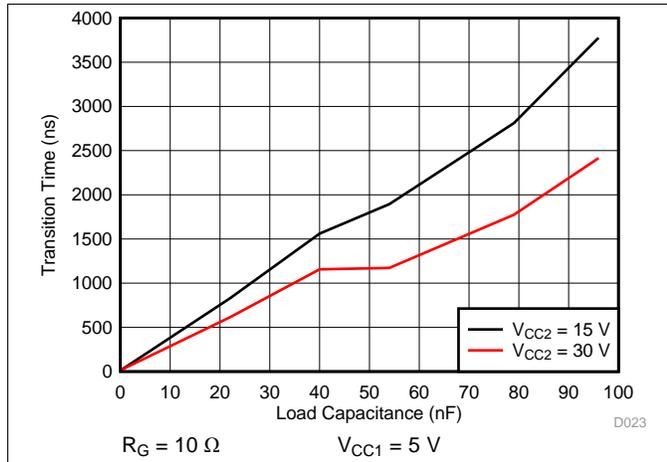
Figure 27.  $t_r$  Rise Time vs Load Capacitance
