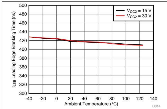
Figure 29. Leading Edge Blanking Time With Temperature
