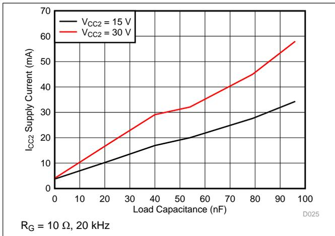
Figure 21.  $I_{CC2}$  Supply Current vs Load Capacitance
