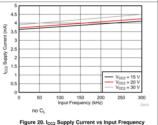
Figure 20.  $I_{CC2}$  Supply Current vs Input Frequency
