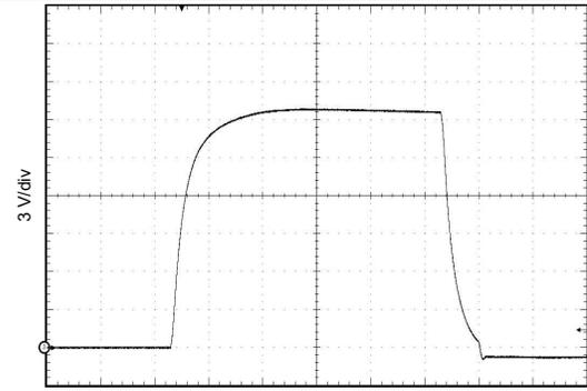
$C_L = 10 \text{ nF}$        $R_G = 10 \Omega$
