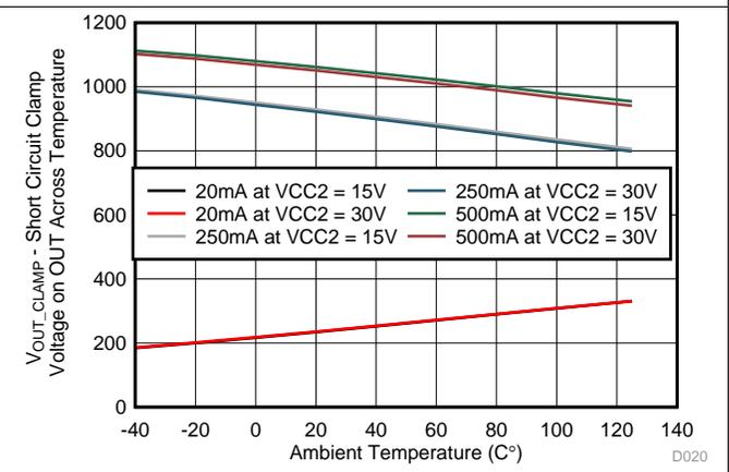
Figure 36.  $V_{OUT\_CLAMP}$  - Short Circuit Clamp Voltage on OUT Across Temperature
