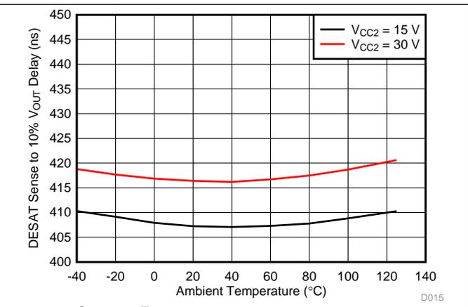
Figure 30. DESAT Sense to  $V_{OUT}$  10% Delay vs Temperature
