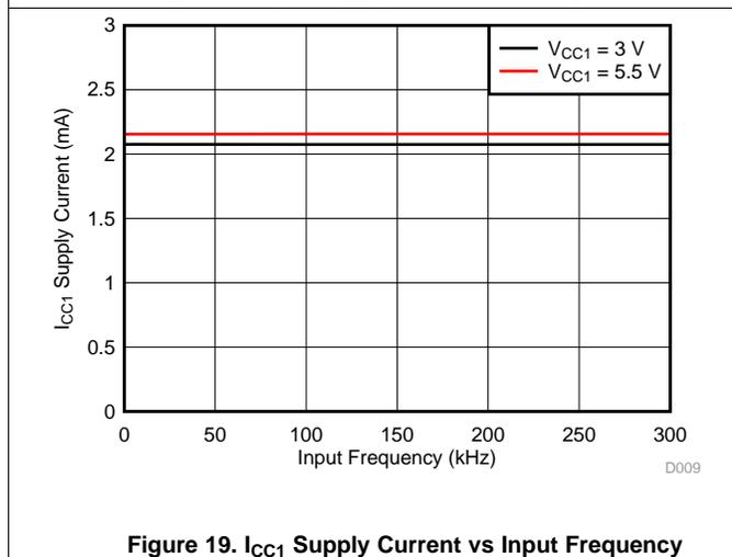
Figure 19.  $I_{CC1}$  Supply Current vs Input Frequency
