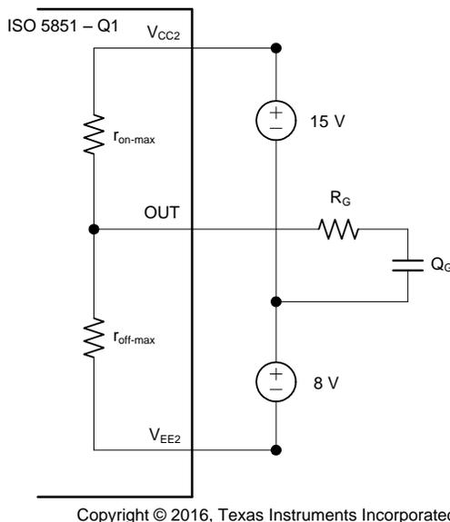
**Figure 50. Simplified Output Model for Calculating  $P_{OL-wc}$**
