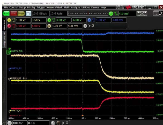
Figure 4-2. Test Results: No Glitch After Increasing Bus Capacitor
