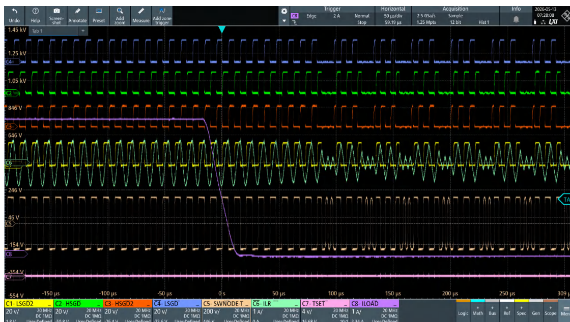
Figure 4-4. Vin = 185V, Vout =12V, Iout = 5A to 0.01A Load Transient (0.2A/us) C1=LO2 Gate Drive, C2= HO1 Gate Drive, C3= HO2 Gate Drive, C4= LO1 Gate Drive C5= Tank Voltage, C6= Tank Current, C7= TSET Pin Voltage, C8 = Load Current
