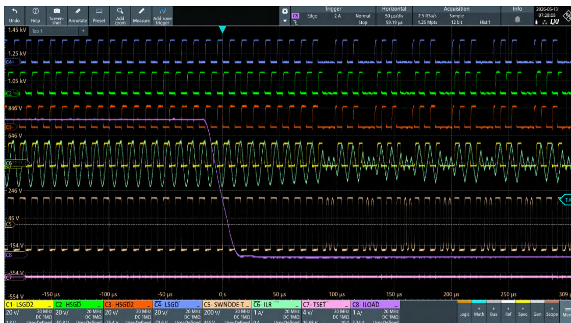
Figure 4-10. Vin = 185V, Vout =12V, Iout = 5A to 0.01A Load Transient (0.2A/us) C1=LO2 gate drive, C2= HO1 Gate Drive, C3= HO2 Gate Drive, C4= LO1 Gate Drive C5= Tank Voltage, C6= Tank Current, C7= TSET Pin Voltage, C8 = Load Current
