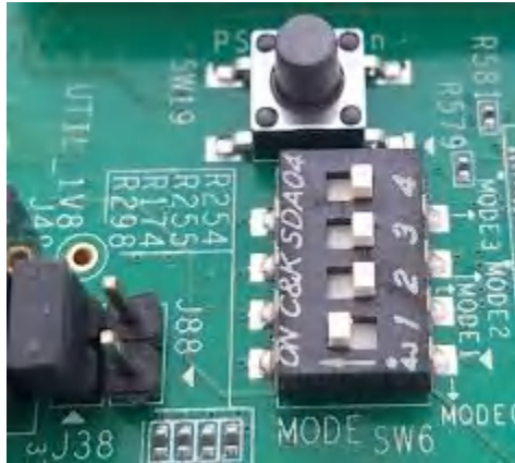
Figure 4-8. Switch State For SD Card Boot
