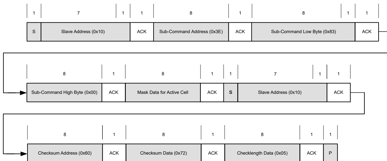
Figure 5-6. Discharge Cell 1 and Cell 3
