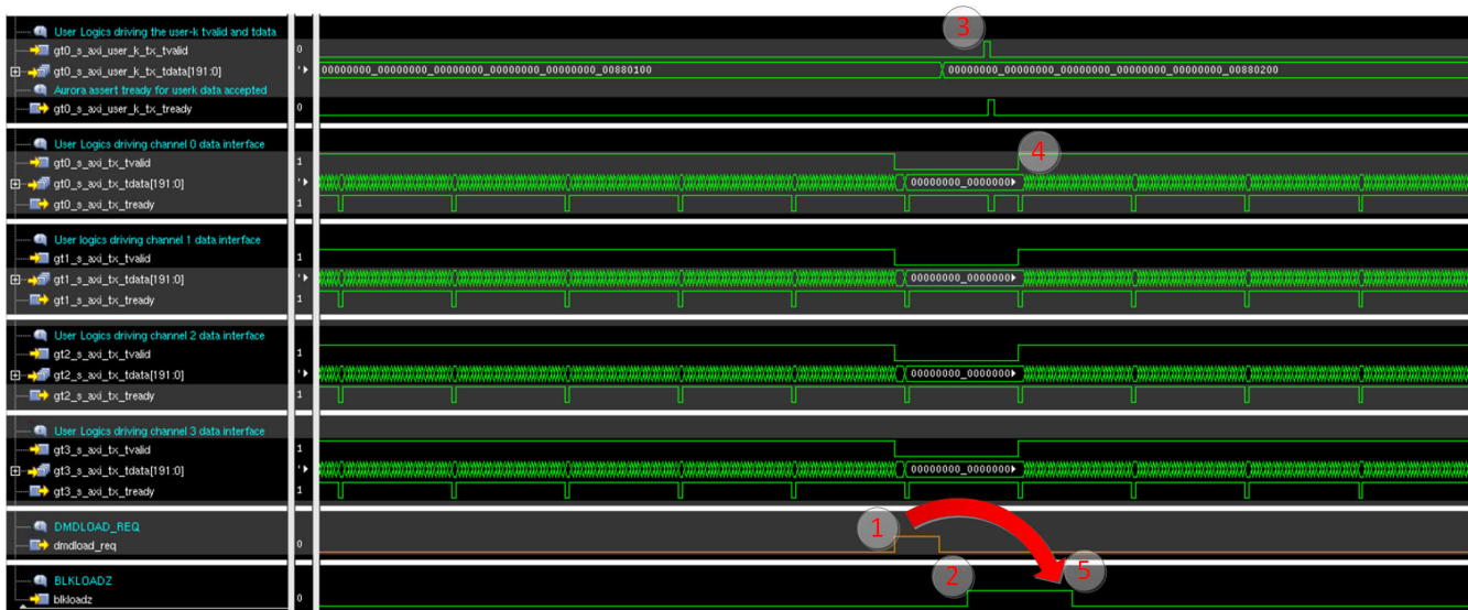
Figure 4-19. End of Block DMDLOAD_REQ Assertion Follow By New Block Control Word Waveform
