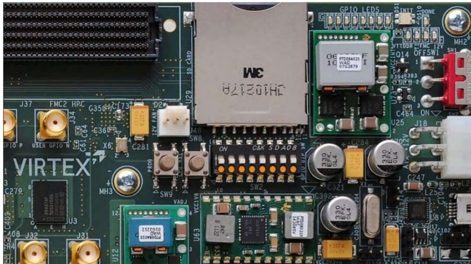
Figure 4-10. GPIO Dip Switches (VC707)
