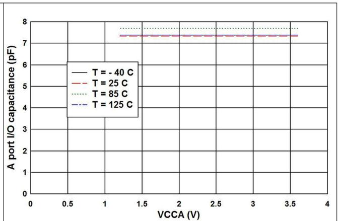
Figure 6-2. Capacitance for A port I/O pins (C<sub>IO</sub>) vs Power Supply (V<sub>CCA</sub>) for V<sub>CCB</sub> = 3.3 V (RUT package)
