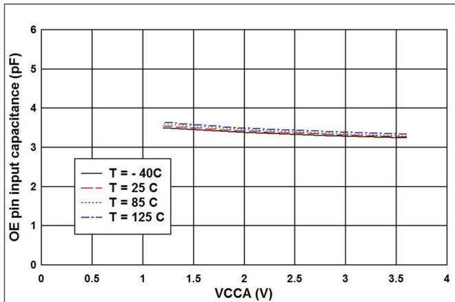
Figure 6-1. Input capacitance for OE pin (C<sub>I</sub>) vs Power Supply (V<sub>CCA</sub>) for V<sub>CCB</sub> = 3.3 V (RUT package)
