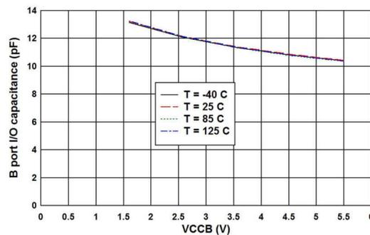
Figure 6-3. Capacitance for B port I/O pins (C<sub>IO</sub>) vs Power Supply (V<sub>CCB</sub>) for V<sub>CCA</sub> = 3.3 V (RUT package)
