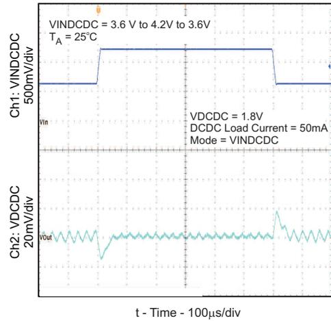
Figure 25. Line Transient Response (DC-DC PWM Mode)
