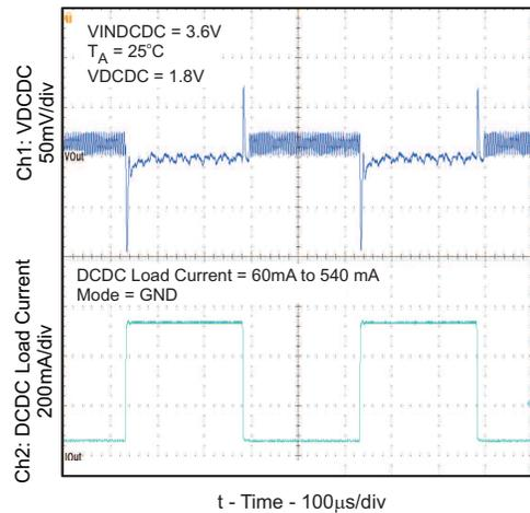
Figure 27. Load Transient Response (DC-DC PFM Mode)
