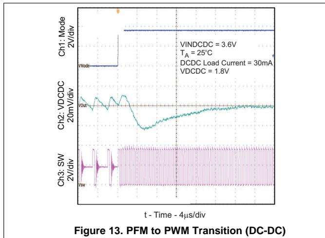
Figure 13. PFM to PWM Transition (DC-DC)
