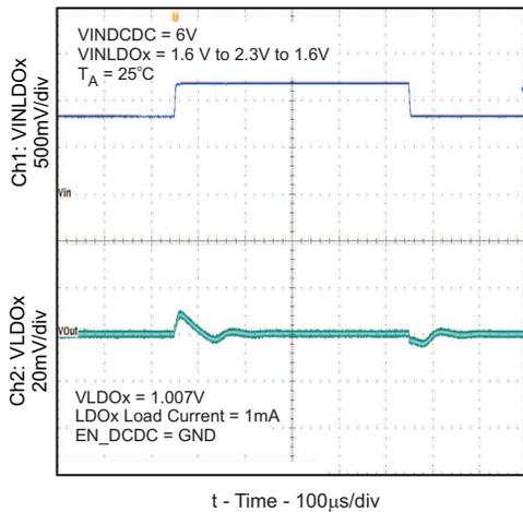
Figure 26. Line Transient Response (LDOx)
