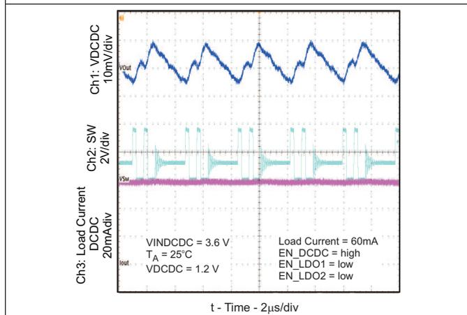
Figure 3. Output Voltage Ripple (DC-DC PFM Mode)
