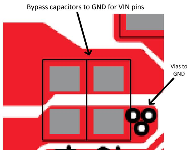
Figure 31. Bypass Capacitor and Via Placement Recommendation
