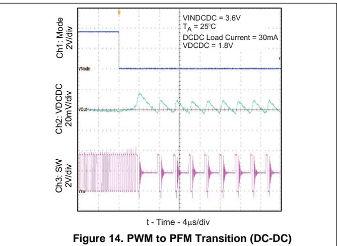
Figure 14. PWM to PFM Transition (DC-DC)
