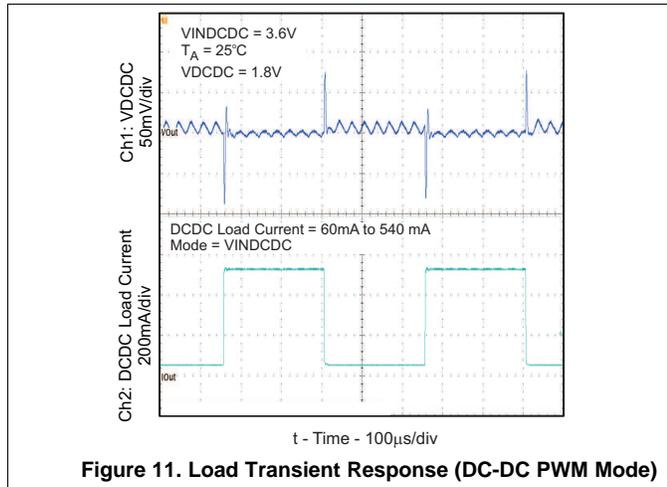
Figure 11. Load Transient Response (DC-DC PWM Mode)
