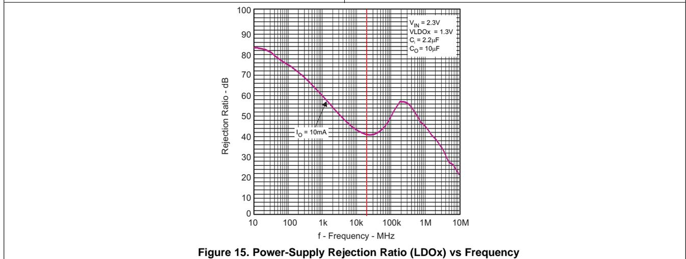
Figure 15. Power-Supply Rejection Ratio (LDOx) vs Frequency
