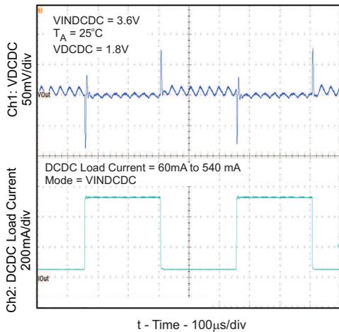
Figure 28. Load Transient Response (DC-DC PWM Mode)
