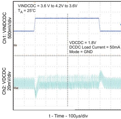
Figure 24. Line Transient Response (DC-DC PFM Mode)
