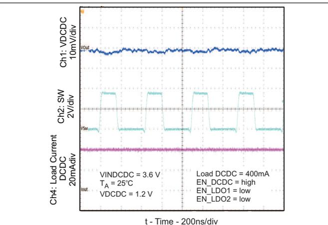
Figure 4. Output Voltage Ripple (DC-DC PWM Mode)
