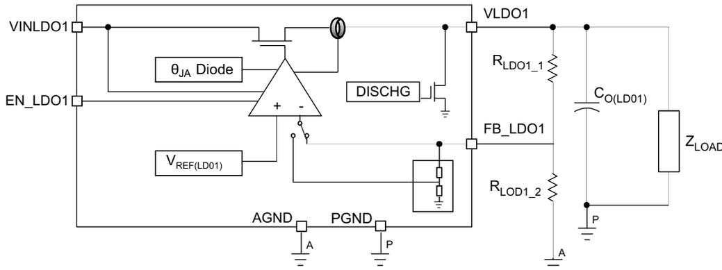
Figure 19. LDO Block Diagram and Output Voltage Setting
