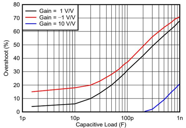
For gain  $\neq 1\text{ V/V}$ ,  $R_F = 1\text{ k}\Omega$ . For gain = 1 V/V,  $R_F = 0\ \Omega$ .
