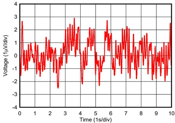
Figure 6-13. 0.1-Hz to 10-Hz Input Voltage Noise
