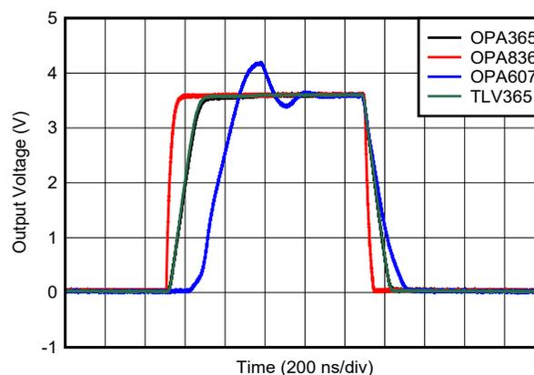
Gain = 10 V/V.  $V_{OUT}$  driven to  $(V-) - 1$  V
