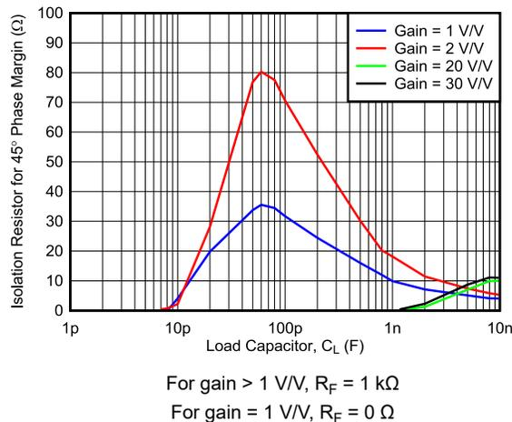
**Figure 7-5. Recommended Isolation Resistor vs Capacitive Load**
