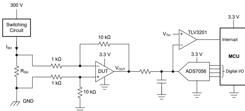
Figure 8-1. Low Side Current Sensing Application Circuit
