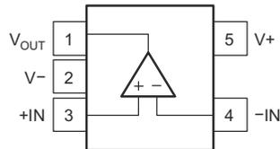
Figure 5-1. TLV365-Q1 DBV Package, 5-Pin SOT-23 (Top View)
