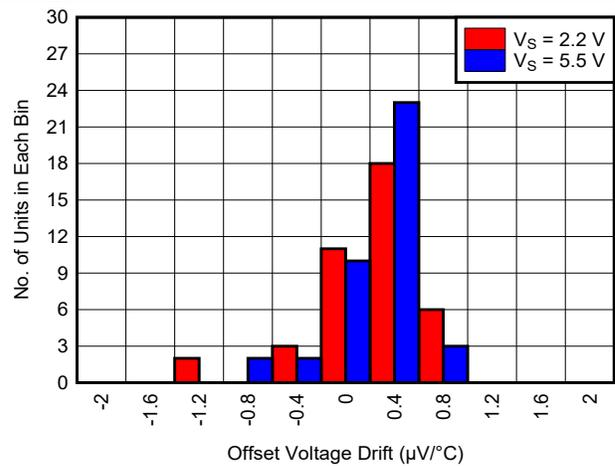
40 units,  $\mu = 0.06\ \mu\text{V}/^\circ\text{C}$ ,  $\sigma = 0.4\ \mu\text{V}/^\circ\text{C}$
