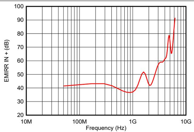
**Figure 6-22. Electromagnetic Interference Rejection Ratio Referred to Noninverting Input (EMIRR<sup>+</sup>) vs Frequency**
