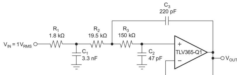
**Figure 7-7. Configured as a Three-Pole, 20-kHz, Sallen-Key Filter**
