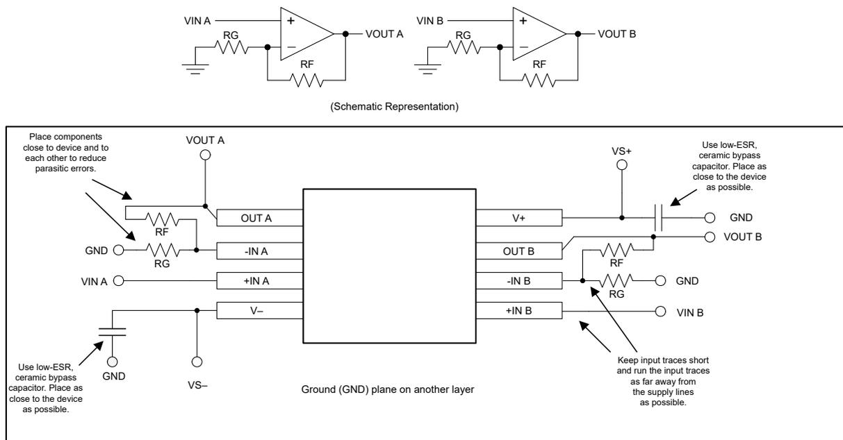
**Figure 8-8. Layout Recommendation for TLV2365-Q1 SOIC Package**
