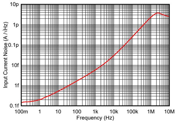
Figure 6-15. Input Current Noise Spectral Density
