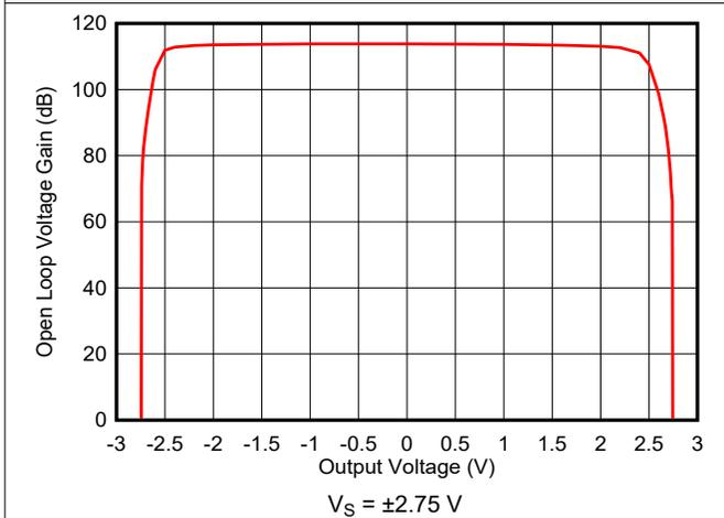
**Figure 6-21. Open Loop Voltage Gain vs Output Voltage**
