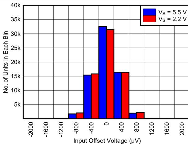
70000 units,  $\mu = 9.3\ \mu\text{V}$ ,  $\sigma = 320\ \mu\text{V}$ .
