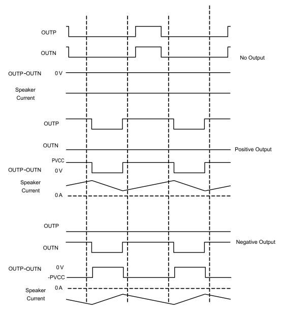
Figure 75. 1SPW Mode Modulation
