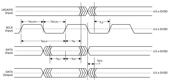
Figure 64. Serial Audio Port Timing in Slave Mode
