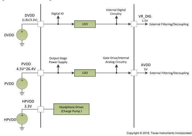
Figure 137. Power Supply Function Block Diagram
