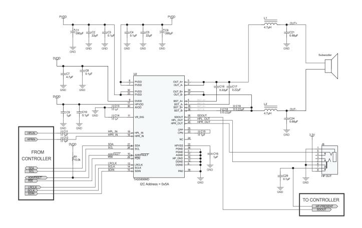
Figure 134. Mono (PBTL) System Application Schematic
