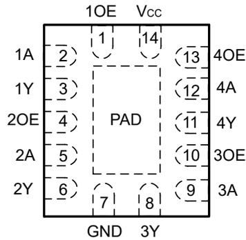
Figure 4-1. BQA Package, 14-Pin WQFN (Top View)
