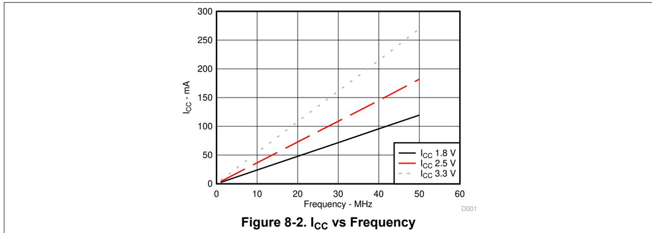
Figure 8-2. I<sub>CC</sub> vs Frequency
