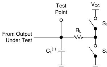
(1) C<sub>L</sub> includes probe and test-fixture capacitance.
