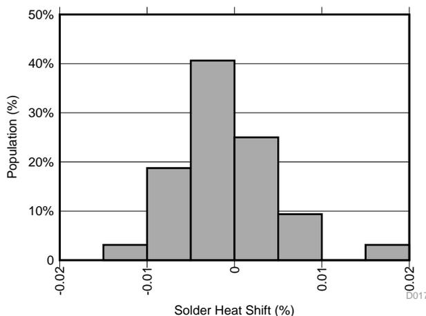
Figure 23. Solder Heat Shift Distribution,  $V_{REF}$  (%)
