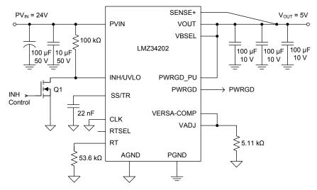
Figure 30. LMZ34202 Typical Schematic
