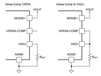
Figure 19. Versa-Comp Configurations
