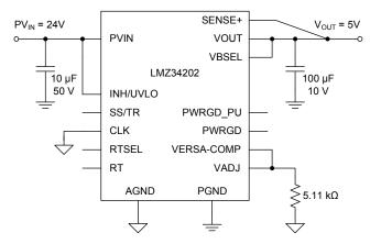
Figure 27. LMZ34202 Minimum External Component Application
