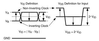
Figure 6-1. Two Different Definitions for Differential Input Signals
