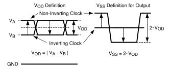
Figure 6-2. Two Different Definitions for Differential Output Signals
