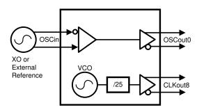
Figure 7-5. Start-Up Clock Using Crystal Reference
