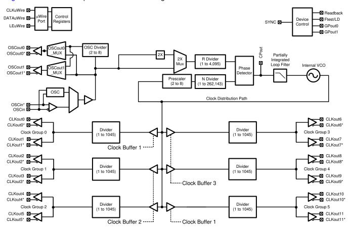
Figure 7-1. Detailed LMK03806 Block Diagram
