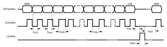
Figure 5-1. MICROWIRE Timing Diagram
