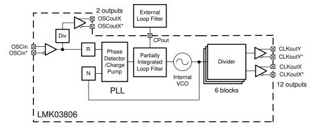
Figure 8-7. Simplified Functional Block Diagram
