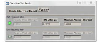
Figure 8-12. PCIe 3.0 RMS Jitter, 100-MHz HCSL
