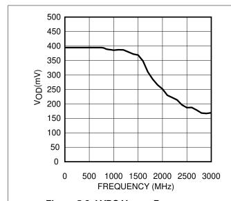
Figure 5-2. LVDS  $V_{\rm OD}$  vs Frequency
