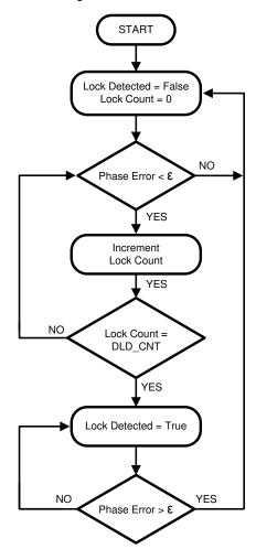
Figure 8-6. Digital Lock Detect Flow Diagram
