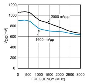
Figure 5-4. LVPECL With 120- $\Omega$  Emitter Resistors  $V_{OD}$  vs Frequency
