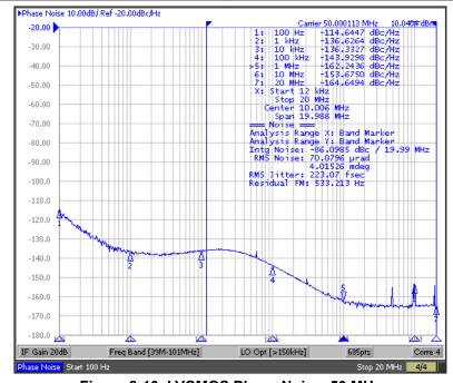
Figure 8-10. LVCMOS Phase Noise, 50 MHz
