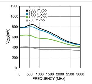
Figure 5-3. LVPECL With 240- $\Omega$  Emitter Resistors  $V_{OD}$  vs Frequency
