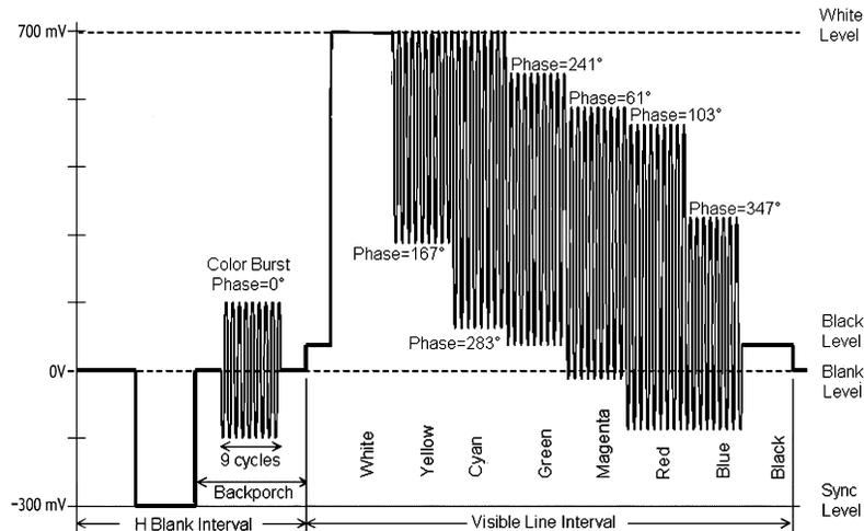
Figure 50. Input Video Signal Before DC Restore Clamp
