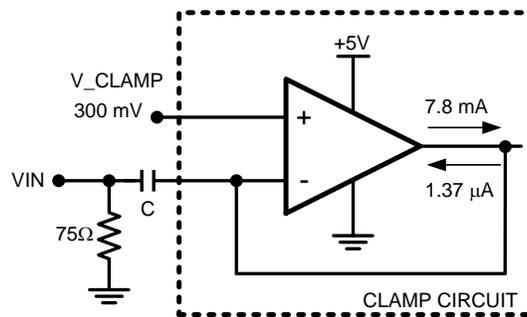
Figure 52. Clamp Circuit
