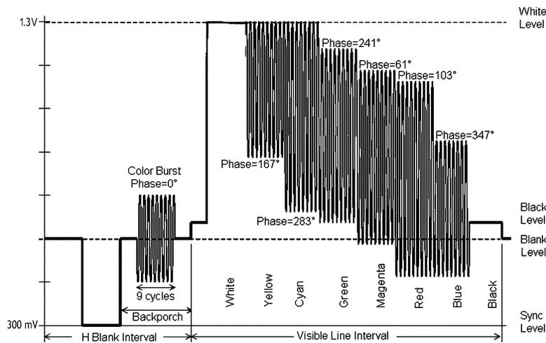
Figure 51. Input Video Signal After DC Restore Clamp
