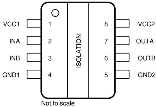
**Figure 4-1. ISO6520 D Package 8-Pin SOIC Top View**
