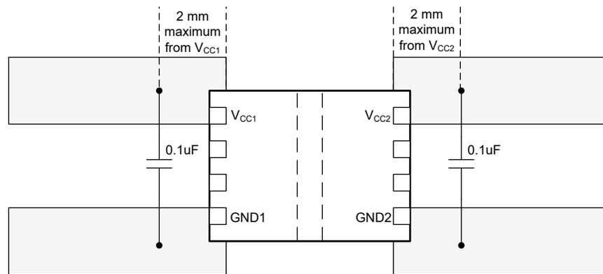
Solid ground islands help dissipate heat through PCB
