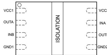
**Figure 4-4. ISO6521 DFN Package 8-Pin REU Top View**
