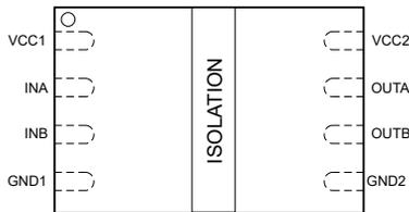
**Figure 4-3. ISO6520 DFN Package 8-Pin REU Top View**
