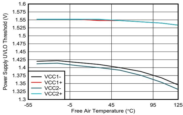
**Figure 5-7. Power Supply Undervoltage Threshold vs Free-Air Temperature**
