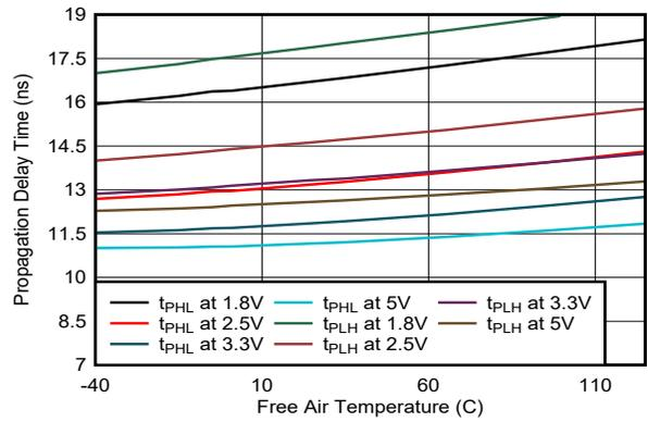
**Figure 5-8. Propagation Delay Time vs Free-Air Temperature**
