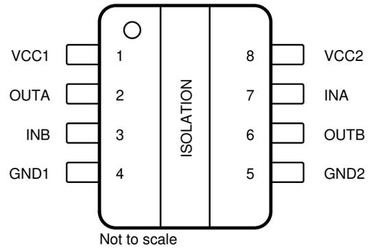
**Figure 4-2. ISO6521 D Package 8-Pin SOIC Top View**
