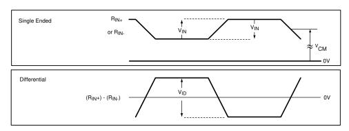
Figure 4-2. FPD-Link III Receiver  $V_{ID}$ ,  $V_{IN}$ ,  $V_{CM}$
