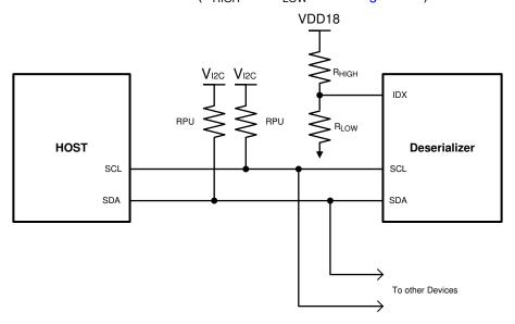
Figure 5-6. Serial Control Bus Connection
