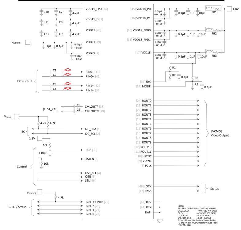
Figure 6-4. Typical Connection Diagram STP
