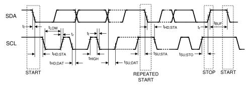
Figure 4-4. I2C Serial Control Bus Timing
