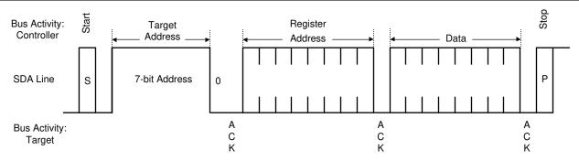
Figure 5-9. Serial Control Bus — WRITE
