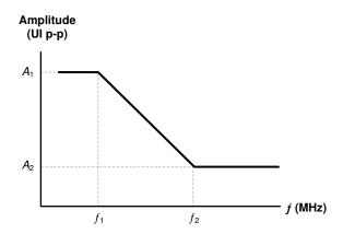
Figure 5-3. Input Jitter Tolerance Plot
