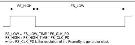
Figure 5-5. Internal FrameSync Signal
