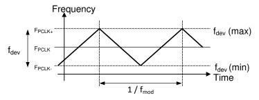
Figure 4-9. Spread Spectrum Clock Output Profile
