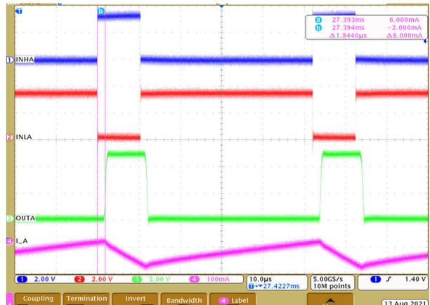
Figure 9-9. Driver delay compensation (1.8 μs)
