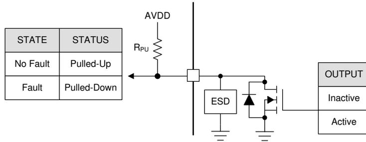
Figure 8-24. Open Drain
