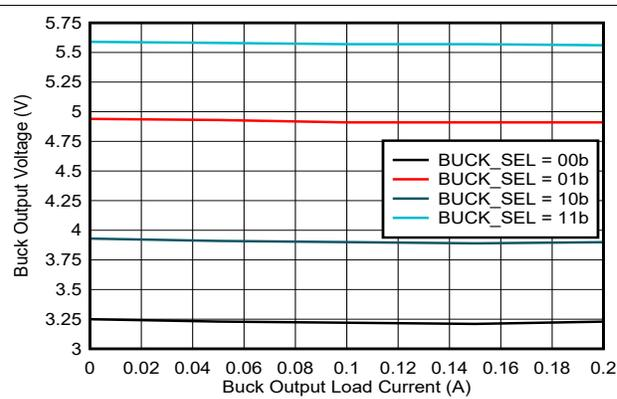
Figure 7-5. Buck regulator output voltage over load current
