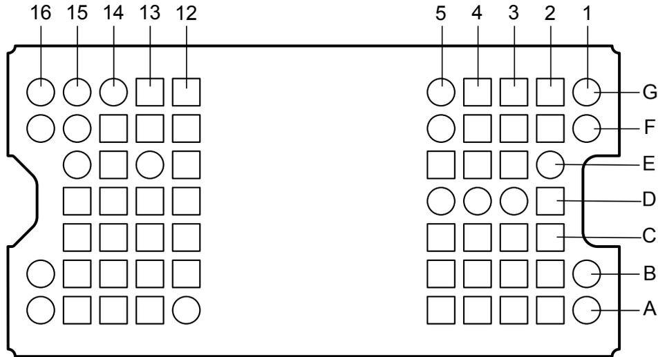
Figure 5-1. FQU Package 64-Pin LGA Bottom View
