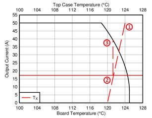
Figure 6-4. Regulating Current to Maintain Safe Operation
