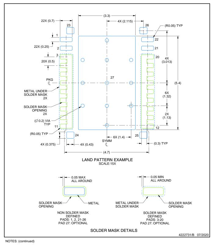
5. This package is designed to be soldered to a thermal pad on the board. For more information, see Texas Instruments literature
