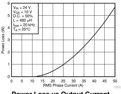
Power Loss vs Output Current
