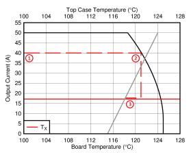
Figure 6-5. Regulate Temperature to Maintain Safe Operation
