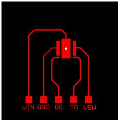
Max  $R_{\theta JA}$  = 50°C/W when mounted on 1 in^2 (6.45 cm²) of 2-oz (0.071-mm) thick Cu.
