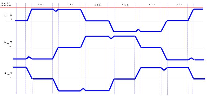
Figure 6-2. Winding Current Waveforms on a BLDC Motor
